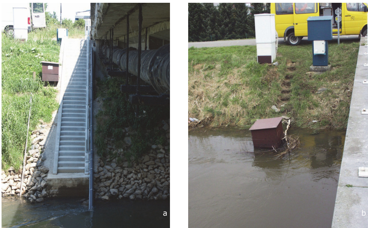
Figure 2.4: Aarschot sediment monitoring location during a) low-flow conditions (5-6-2008) and b) high-flow conditions (2-3-2004) leading to the inundation of the construction containing the SIGMA 900 sampler.
