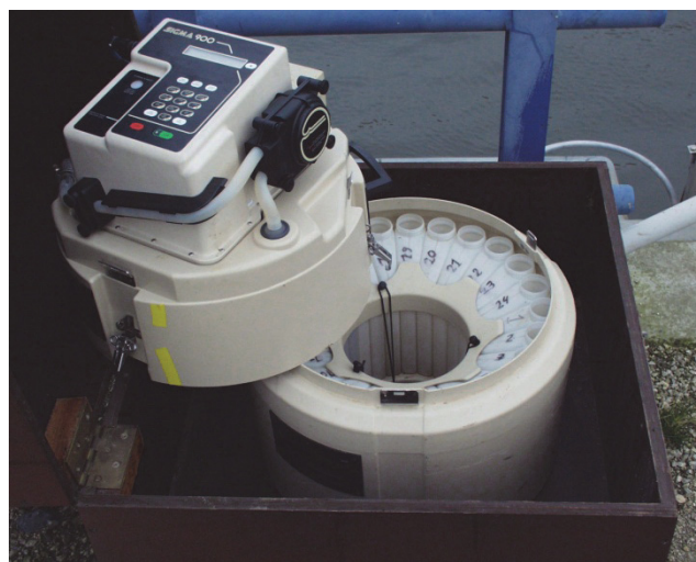
Figure 2.3: Unrefrigerated SIGMA 900 automatic pumping sampler, with 24 bottles
