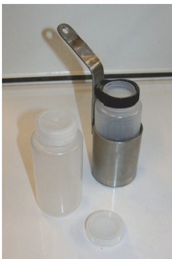
Figure 2.2: Weighted-bottle sampler as constructed by FHR
