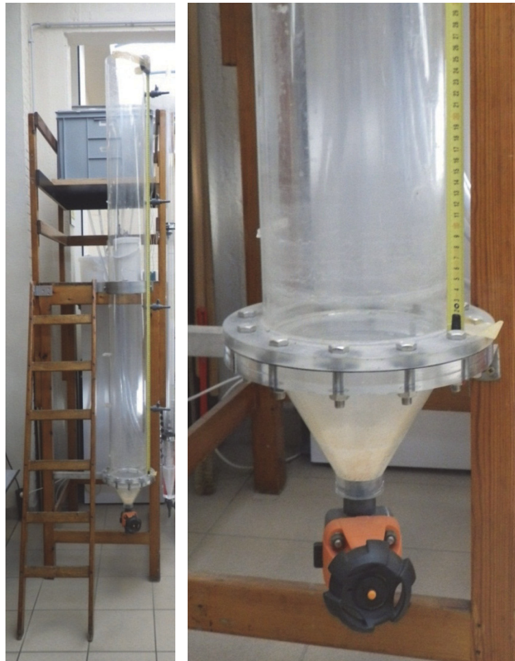
Figure 3.5: Settling tube constructed in FHR's sedimentological laboratory
