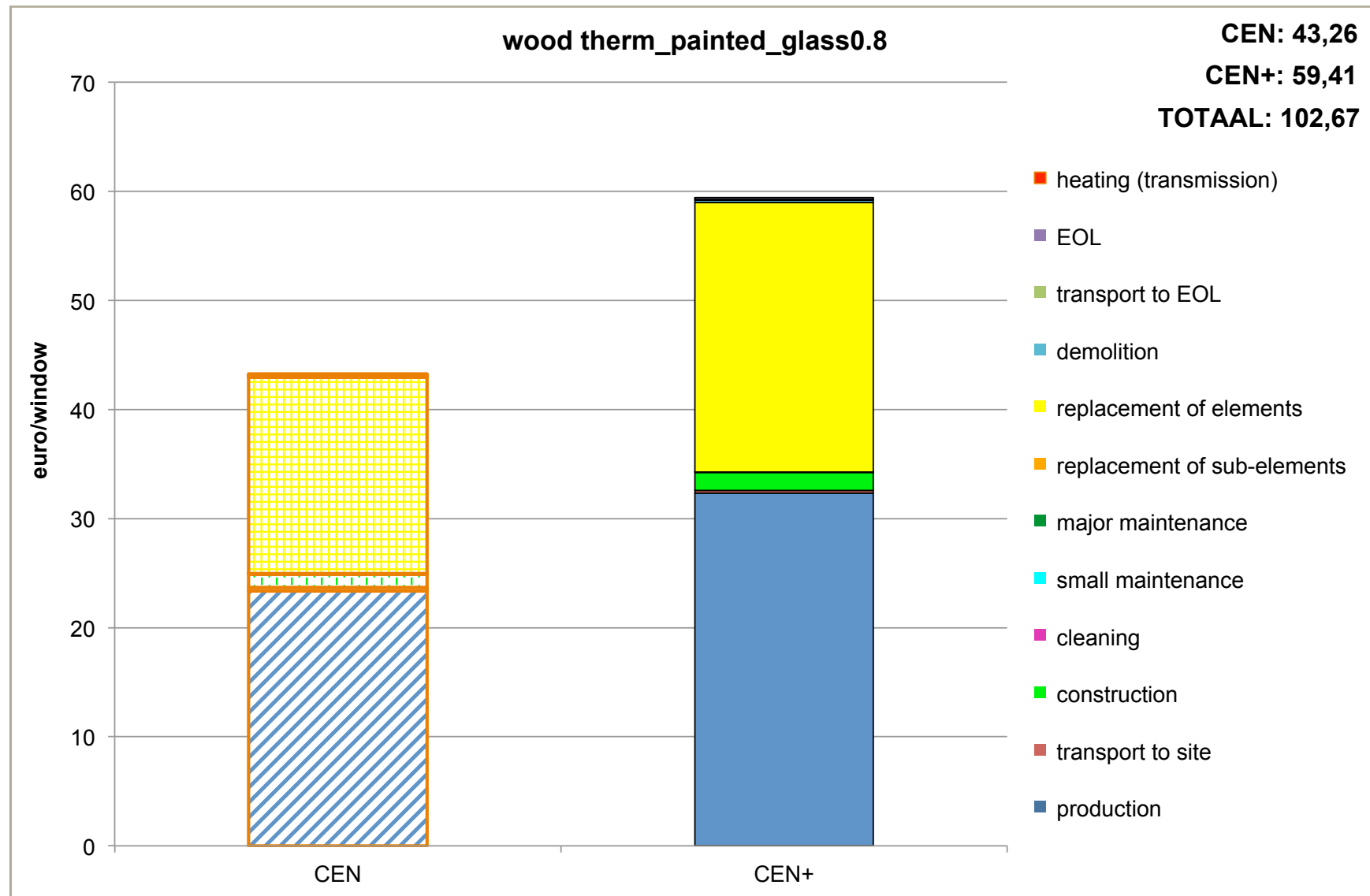
Figure window 8.9.1: Aggregated environmental profile (divided into CEN and CEN+) of variant 'wood therm_painted_glass0.8' per life cycle stage, expressed in monetary units.
