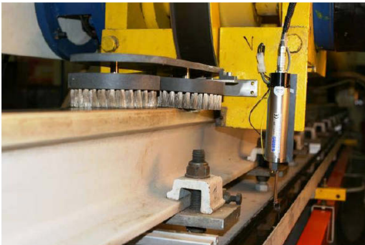
a. Monitoring the rail's position
