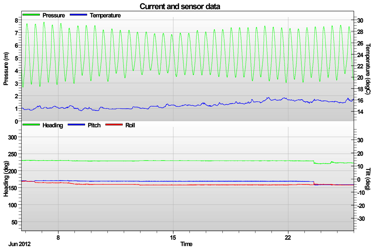
Figure 9 – Temperature, pressure and data regarding positioning recorded by Aquadopp 2, 2012.
