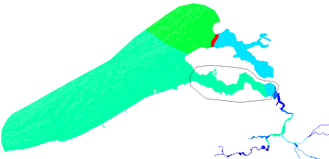
Figure 141 – Bed roughness field of the Scaldis model (the polygon indicates the area where the bed roughness is adapted)
