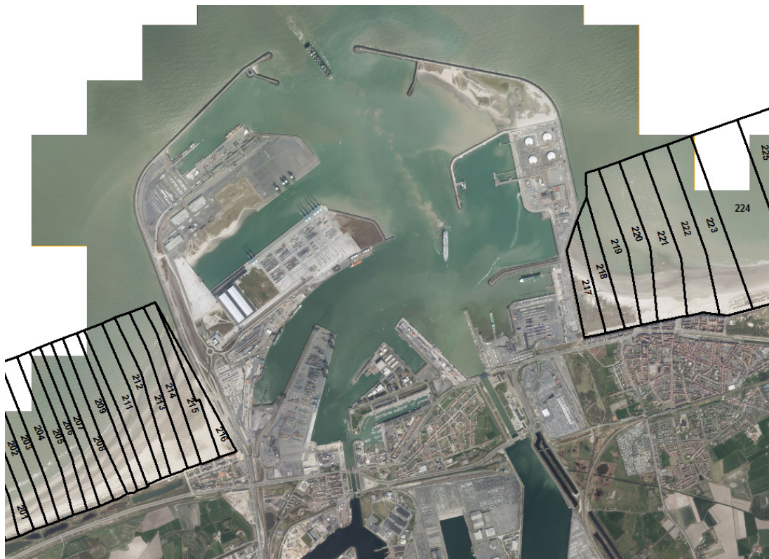
Figure 36 – Volume calculation limits for the sections near Zeebrugge Harbour.
