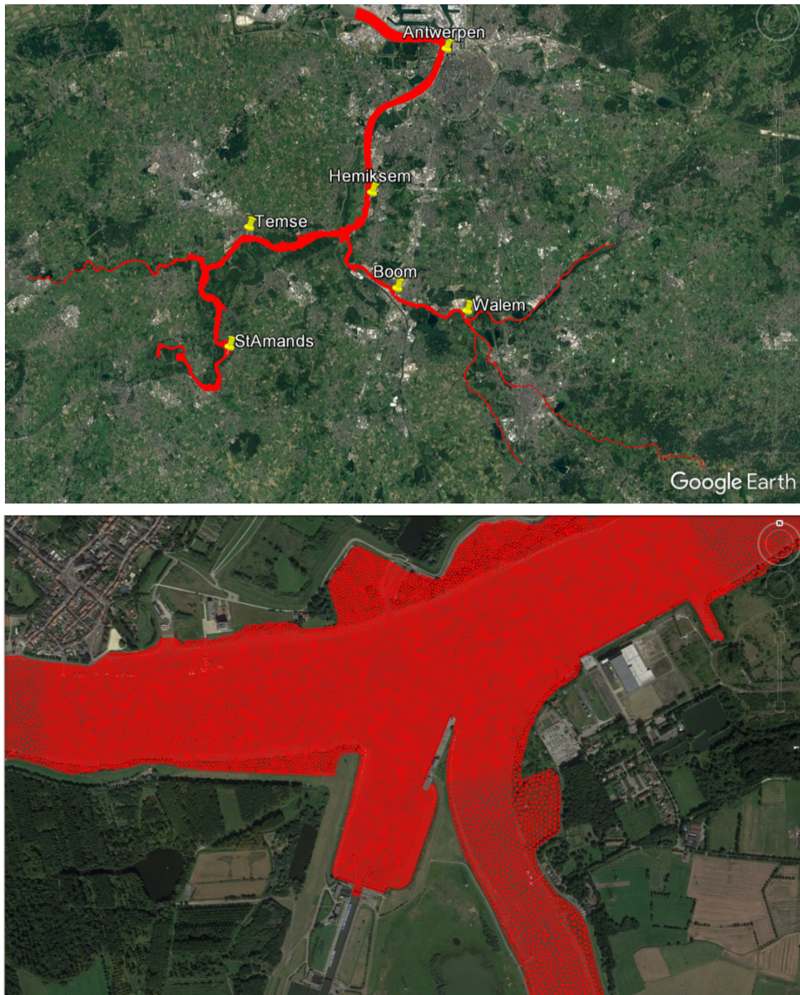
Figure 22 – Overall grid of the Wintam model (upper) and zoom in to the Wintam lock (lower).
