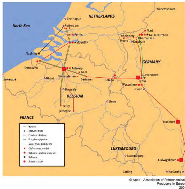
Figure 42: Major refining, steam-cracking operations and related pipelines in Northwest Europe (Source: Petrochemicals Europe)
