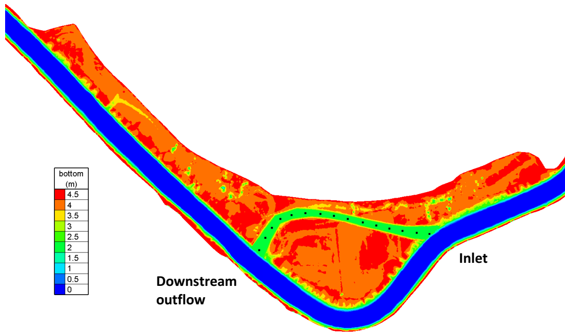
Figure 17 – The points along the thalweg of the secondary channel in the scenario A
