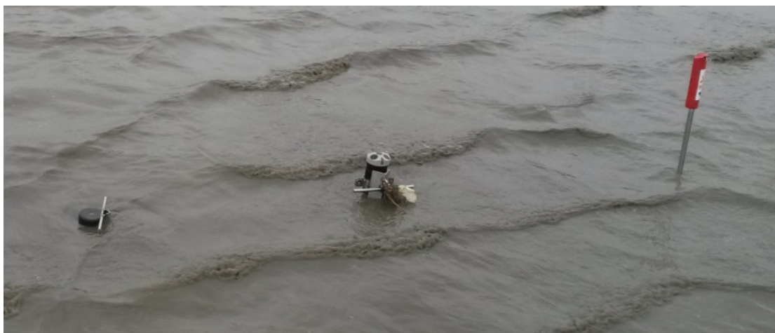
Figure 3-3 – Pressure sensor (left), ADCP (middle) and sedsensor (right) on the low mudflat
