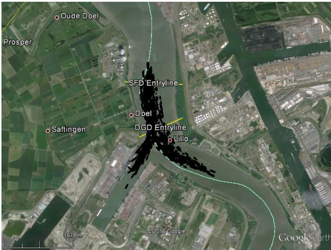
Figure 5-1 – Traces of ships that cross the two considered entry lines, north (SFD) and south (DGD), during tidal cycle 5 (31/10/2015 12:42 – 01/11/2015 00:56), as produced by the FHR tool.
