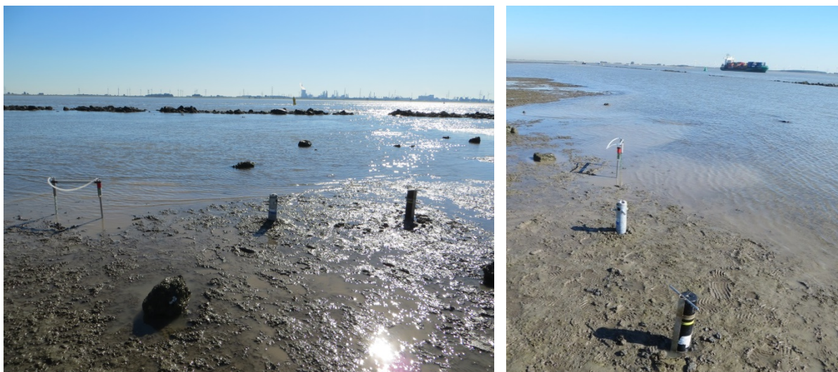
Figure 3 – Measurement instruments (NIOZ sedsensor, Aquadopp ® and pressure sensor) at Saeftinghe-South location
