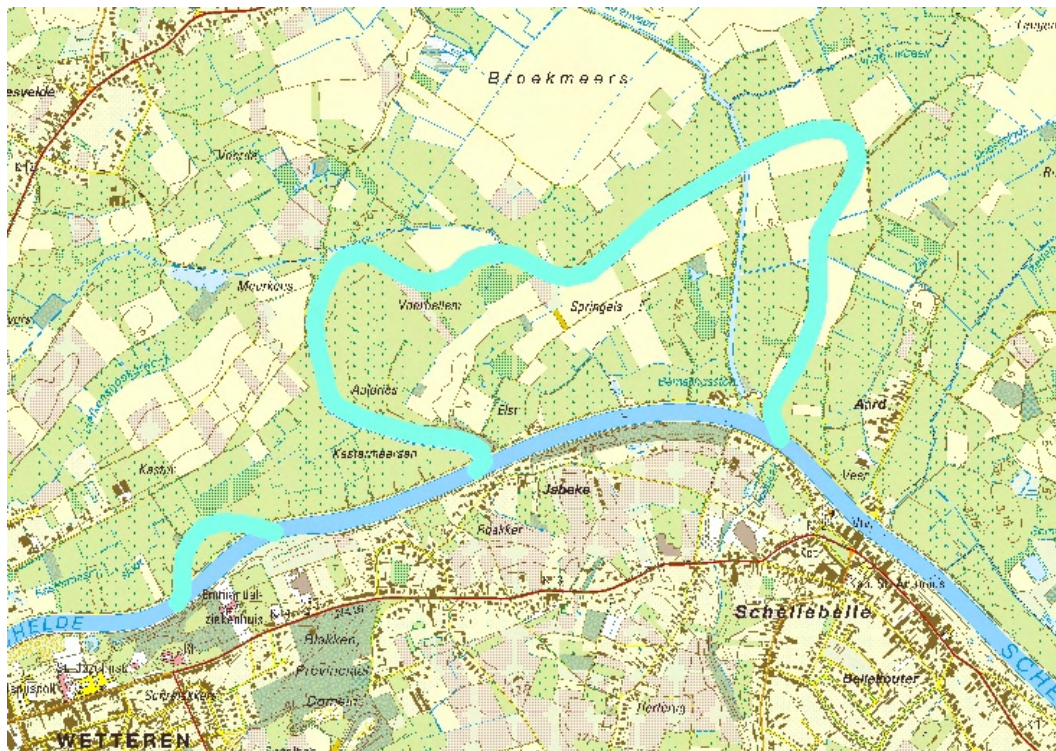
Figuur 3.71 Rechttrekkingen in de Kastermeersen en Kalkense Meersen (Wetteren-Schellebelle) / Canalization in the Kastermeersen and the Kalkense meersen near Wetteren and Schellebelle
