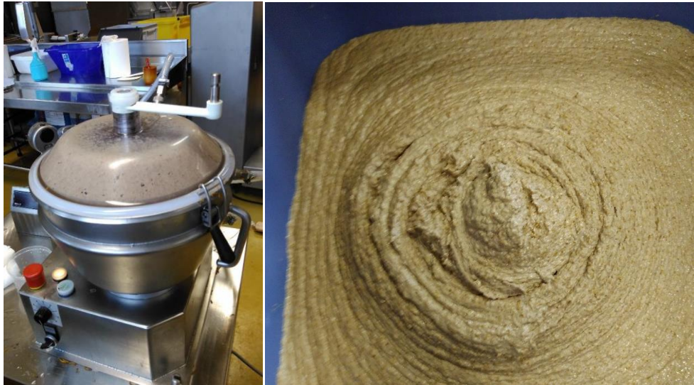
Figuur 26: Links: Schotelcutter (Stephan UM 12, A. Stephan); Rechts: meelwormenpasta (Lab4Food, 2017)
