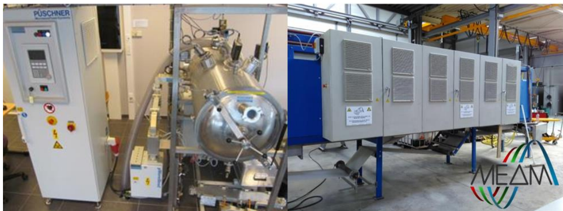
Figure 24: left: µWave Vac0350 batch microwave dryer (Püschner); right: MEAMDRY S 32 belt microwave dryer with 16 sources of 2 kW and a conveyor length of 4 m (MEAM) (VIVES, 2017)
