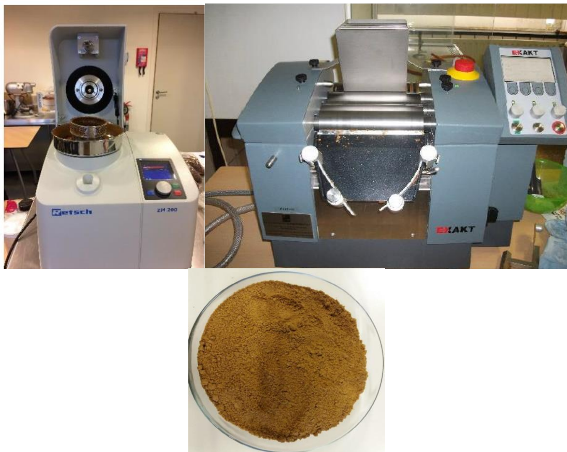
Figure 28: equipment ILVO; top left: Retsch mill (ZM 200, Retsch); top right: three roll mill (EXAKT, Three Roll Mill 80E, E&R); bottom: mealworm meal (Lab4Food, 2017)
