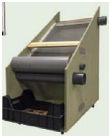
Figure 3: mechanical beetle separator (Inagro, 2020)
