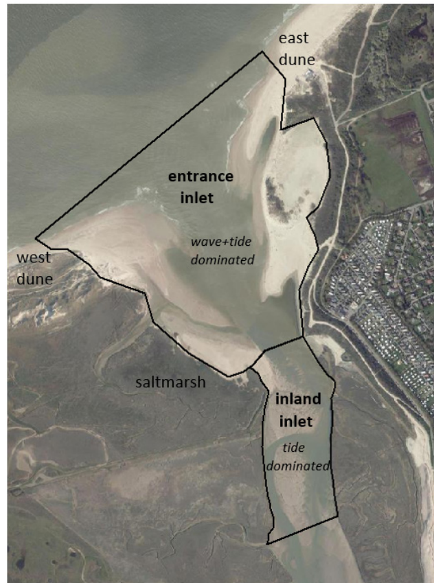
Figure 4 – Morphological units of the tidal inlet. Unit delineated based on the 5m contour line.
