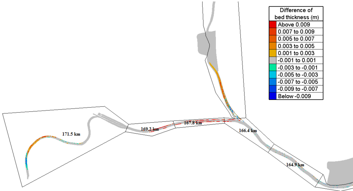
Figure 145 – Difference of bed thickness in Upper Sea Scheldt (165 km – 171 km) in 2050_VaG_AminCL
