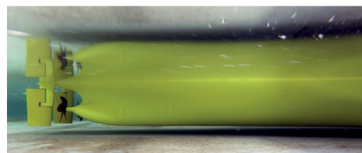
10% UKC test at Towing Tank for Manoeuvres in Confined Water
