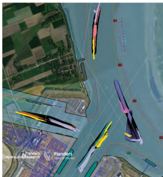
Figure 66 – Scenario U5 with four ULCS at short distance from each other on the four stretches around the DGD mouth
