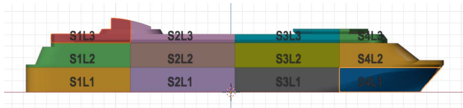
Figure 30 – Sideview of the hull of the WINDLASS cruise ship REF divided in four sections and three layers.
