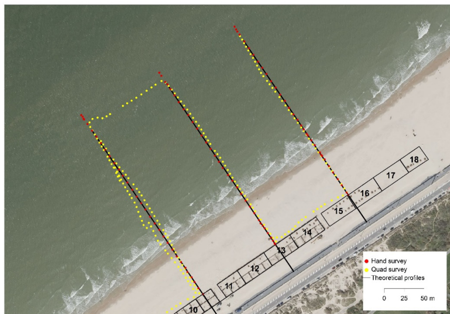
Figure 11 – Maps of A) raw and B) re-projected point surveys for both hand RTK-GPS and quad systems (Profile 4, 5, 6).
