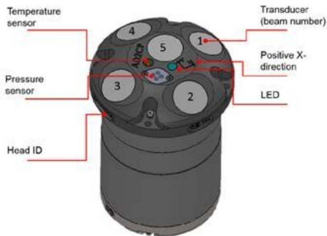
Figure 22 – A) Example of frame used for the campaign, B) Sketch of the ADCP Nortek Signature 1000
