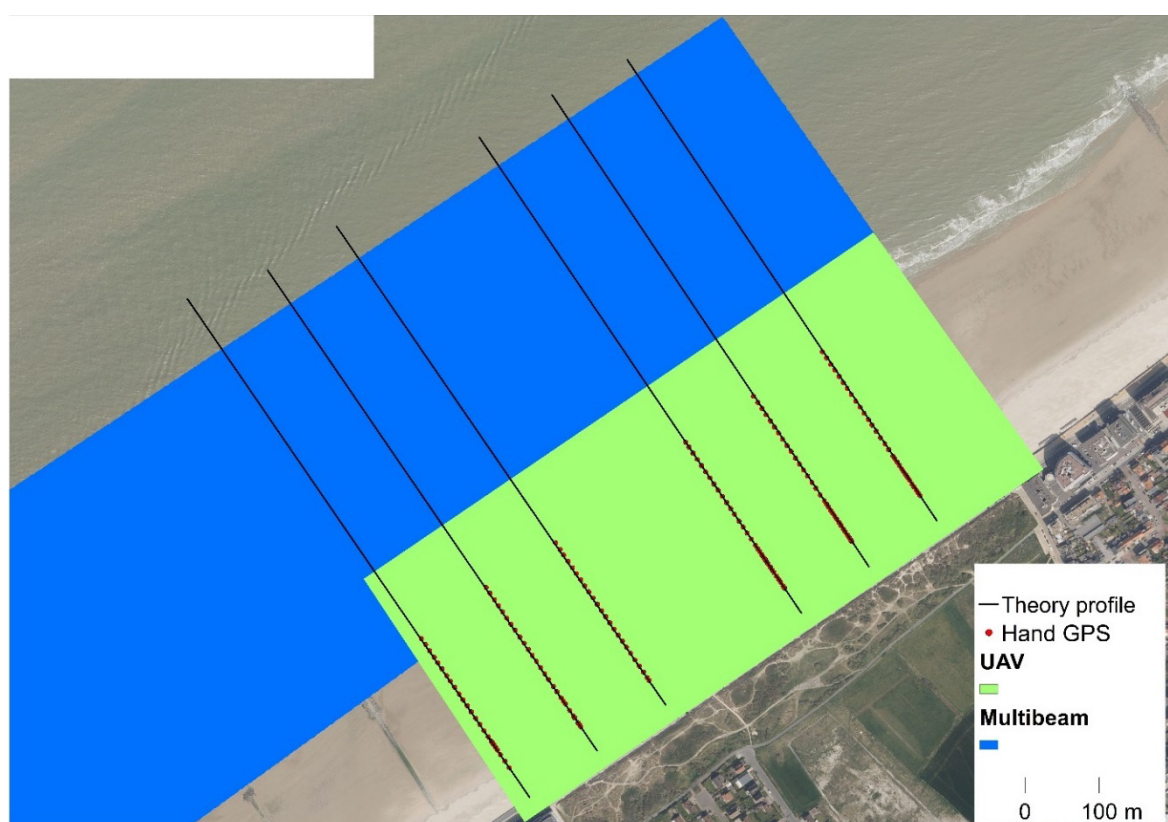
Figure 17 – Areas of the different survey techniques on 12/09/2022. Profile 1 (left) to profile 6 (right).
