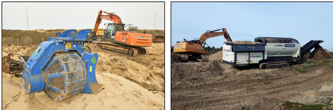
Figure 44. Left: a rotary sieve bucket for an excavator (Y. Adams). Right: an autonomously driving drum sieve (K. Lesage).
