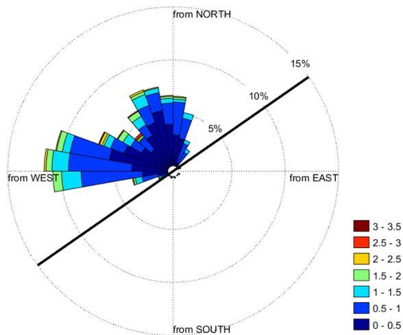
Figure 34 – Wave rose at Raversijde wave buoy during the period July 2014 – July 2017.
