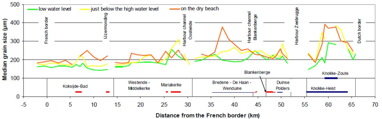
Figure 35 – Longshore variation of the median grain size for three positions on the beach (after Deronde, 2007).
