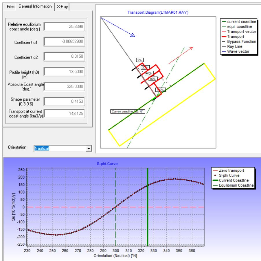
Figure 38 – Relation between coast angle and sediment transport (S-Phi curve) for run MAR01.
