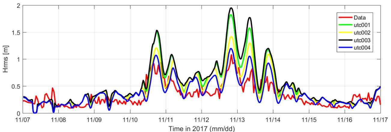
Figure 45 – Comparison of measured and computed wave height.
