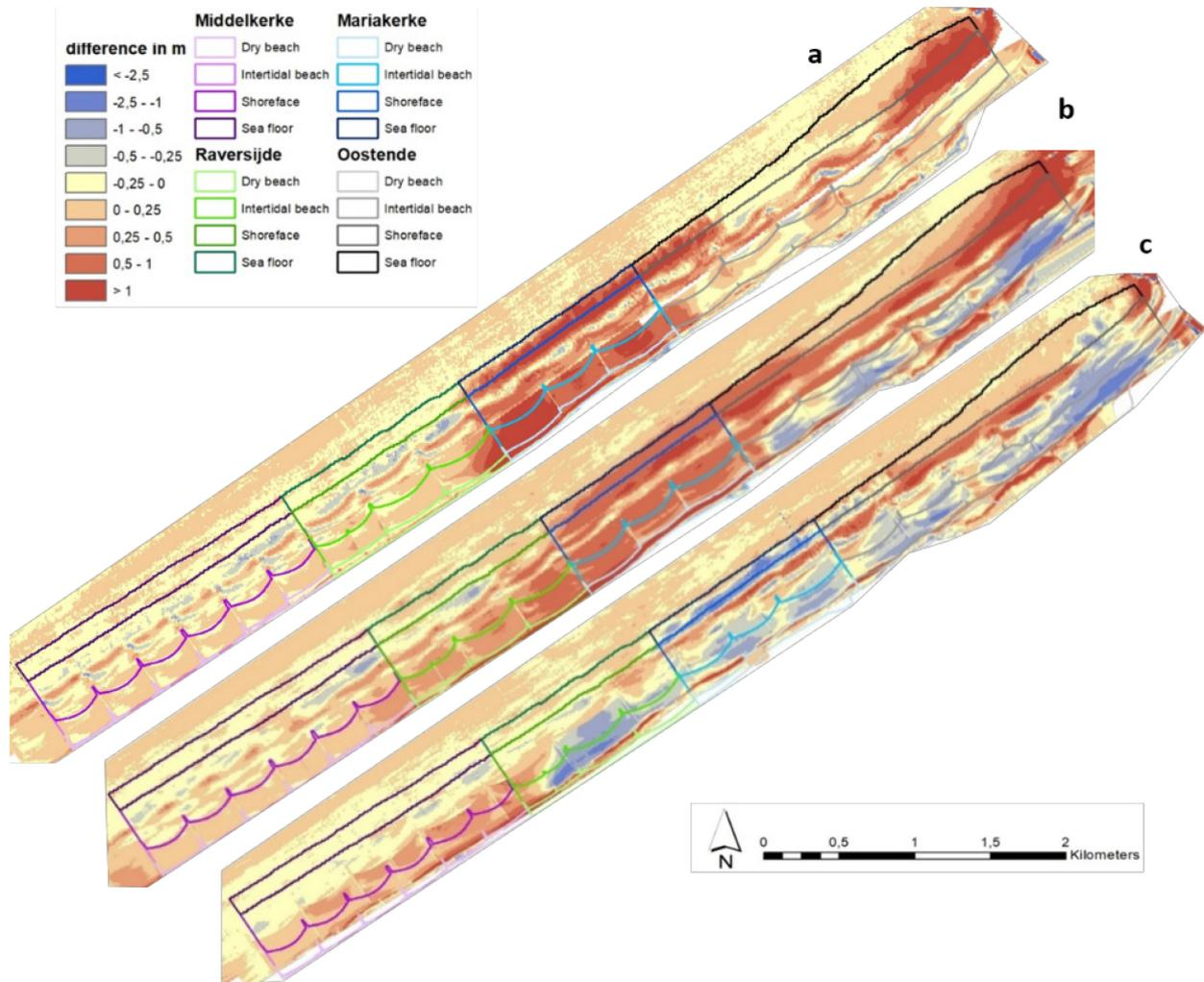
Figure 11 - The digital elevation model difference between different years: a) difference between 2014 and 2013; b) difference between 2013 and 2017; c) difference between 2014 and 2017.
