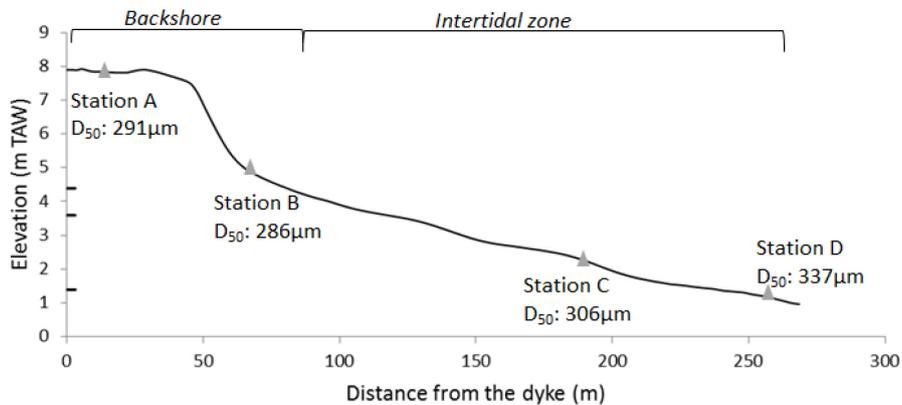
Figure 36 – Sediment characteristics across the beach topography
