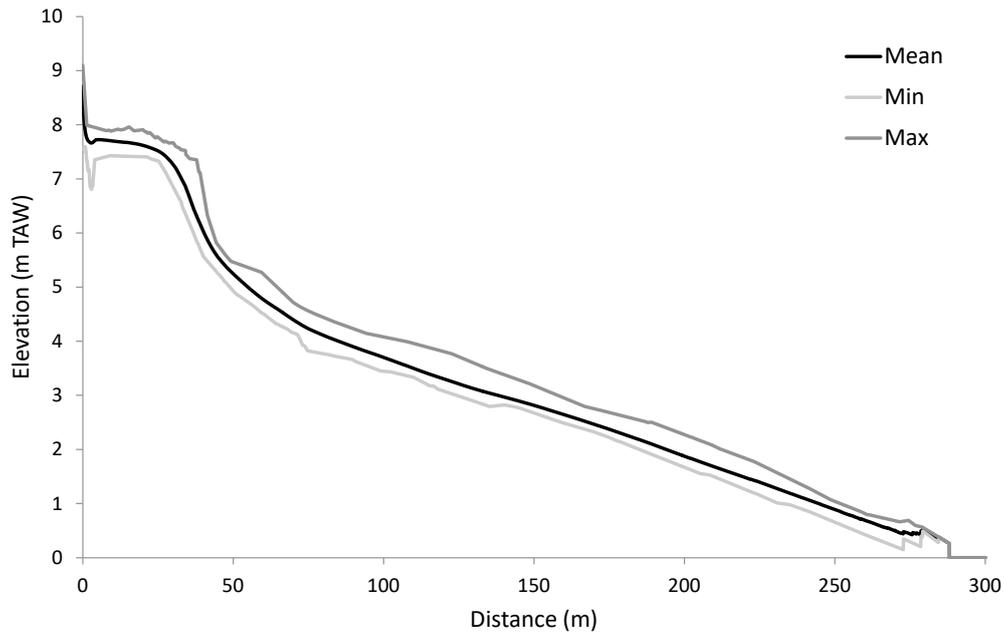
Figure 6 – Envelope of the cross-shore profiles for section P104 (a, b, c) at Mariakerke from September 2015 to December 2017.
