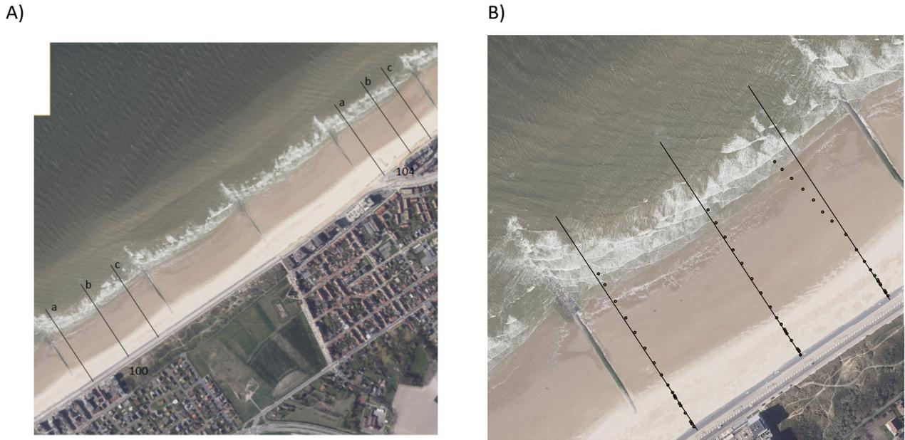
Figure 4 – A) Map of the location of the cross-shore referenced profiles; B) Example of observed shift of a profile.
