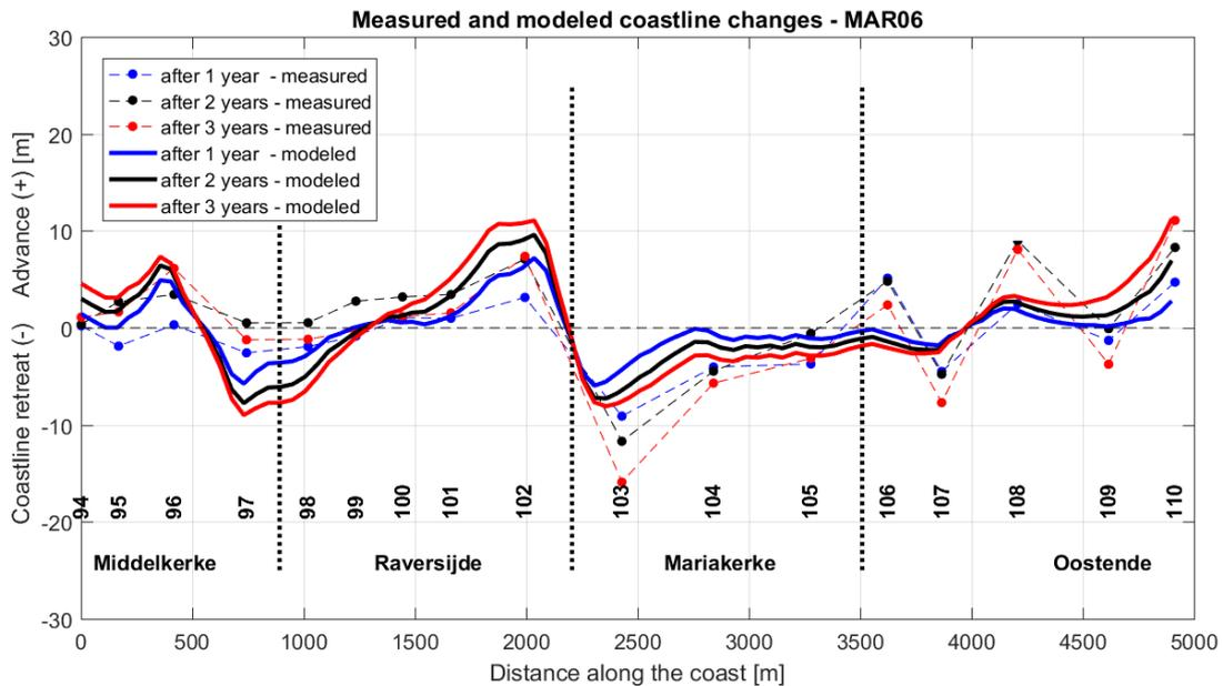
Figure 40 – Modeled vs. measured coastline changes after 3 years.
