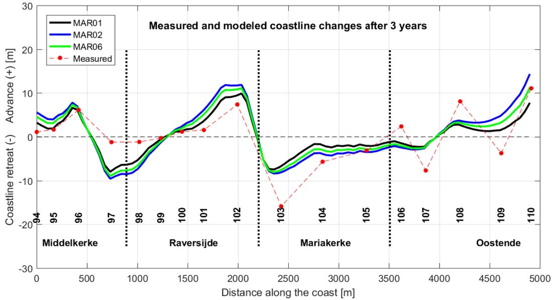
Figure 39 – Modeled vs. measured coastline changes after three years.
