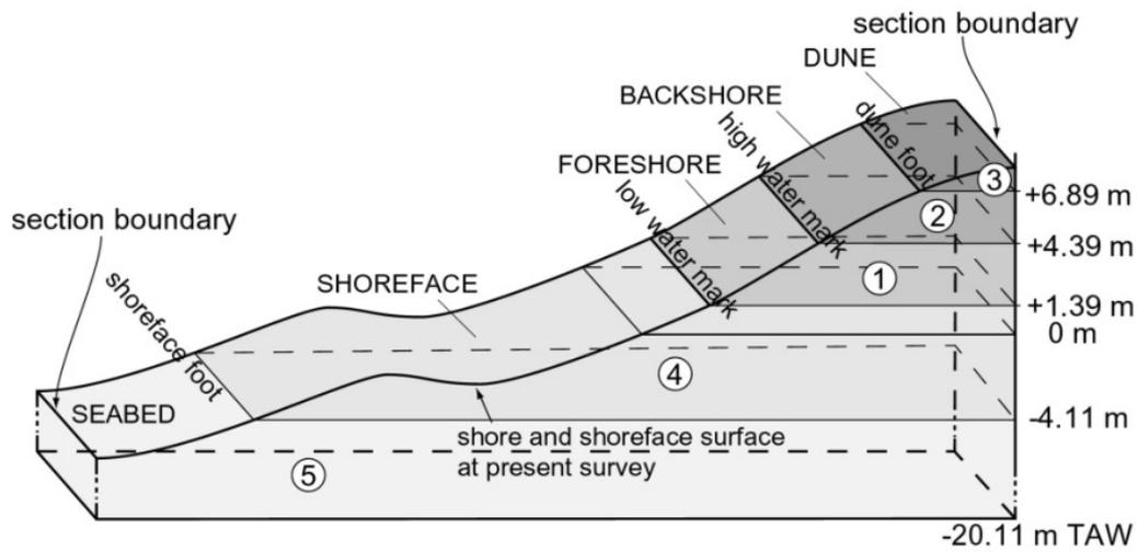
Figure 7 - Schematic representation of the cross-shore divisions at the Belgian coast (after Houthuys, 2012).
