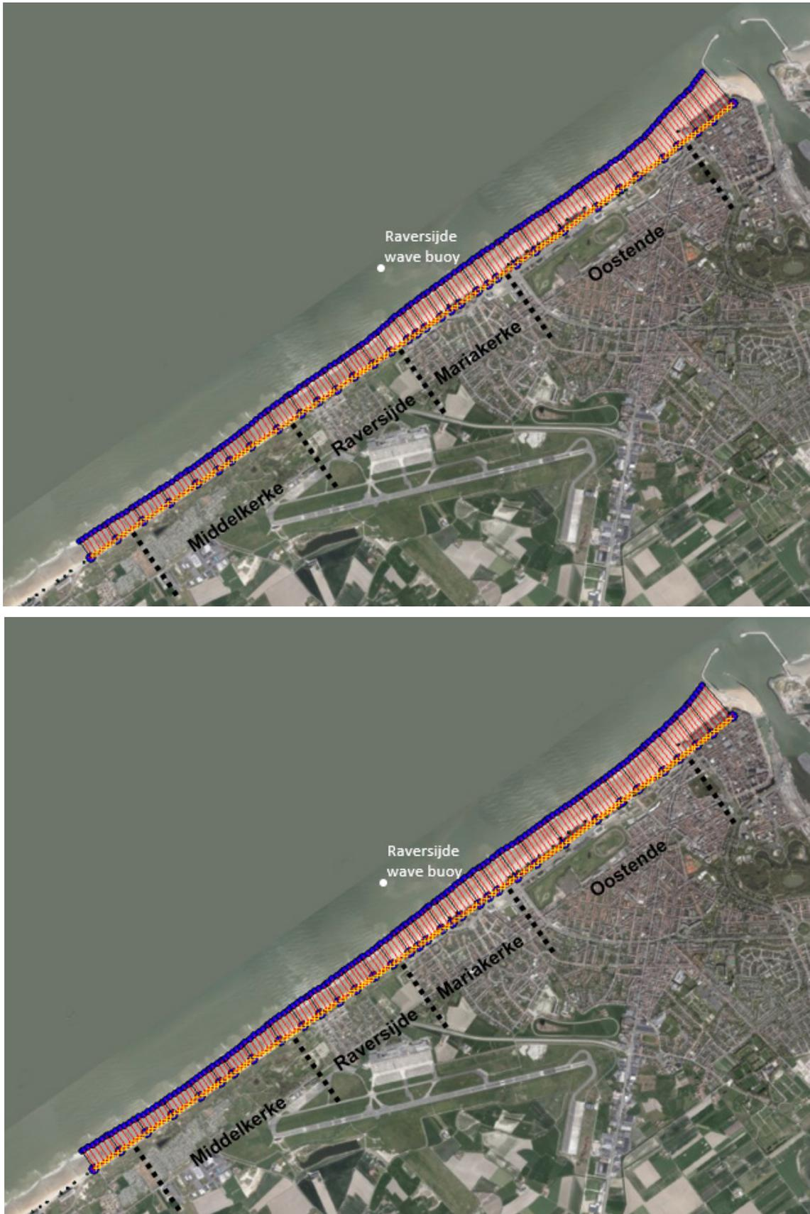
Figure 37 – Unibest-CL model grid and initial coastline (2014) for calibration runs (upper) and (2018) for prediction run (lower).
