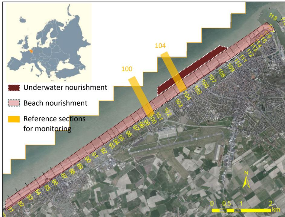
Figure 1 - Pilot site for shoreface nourishment test, Mariakerke coastal area and the reference sections.
