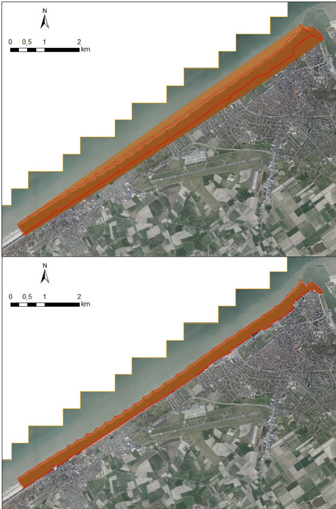
Figure 49 - Example of the delineated polygon over the interpolated DEM (above) and clipped DEM (below) (survey conducted in 27/10/2015).
