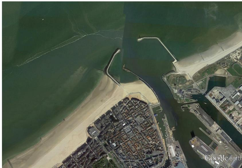
Figure 24 – The submerged (during high tide) groin attached to the southern jetty of the Ostend port which is trapping large volumes of sand (Google Earth 2019).
