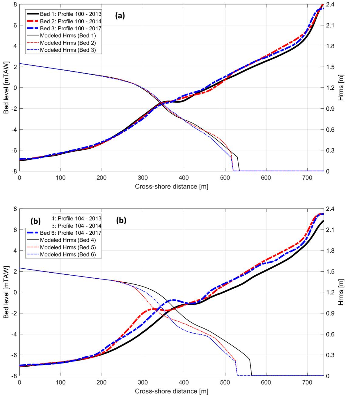
Figure 47 – Modeled  $H_{rms}$  with (a) profile 100 (without, soon after and three years after beach nourishment) and (b) profile 104 (without, soon after and three years after beach & shoreface nourishment) - Low water.
