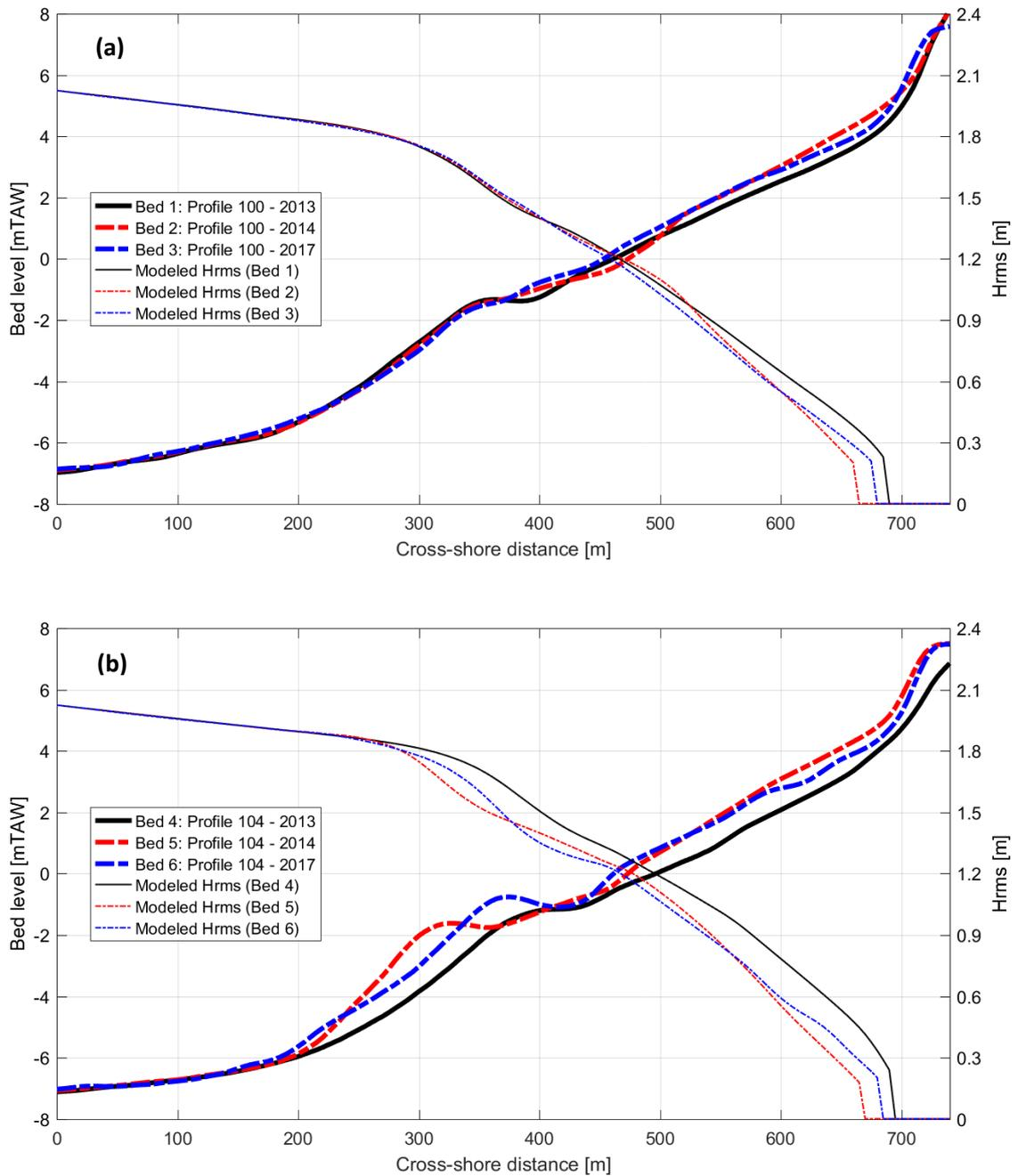
Figure 46 – Modeled  $H_{rms}$  with (a) profile 100 (without, soon after and three years after beach nourishment) and (b) profile 104 (without, soon after and three years after beach & shoreface nourishment) - High water.
