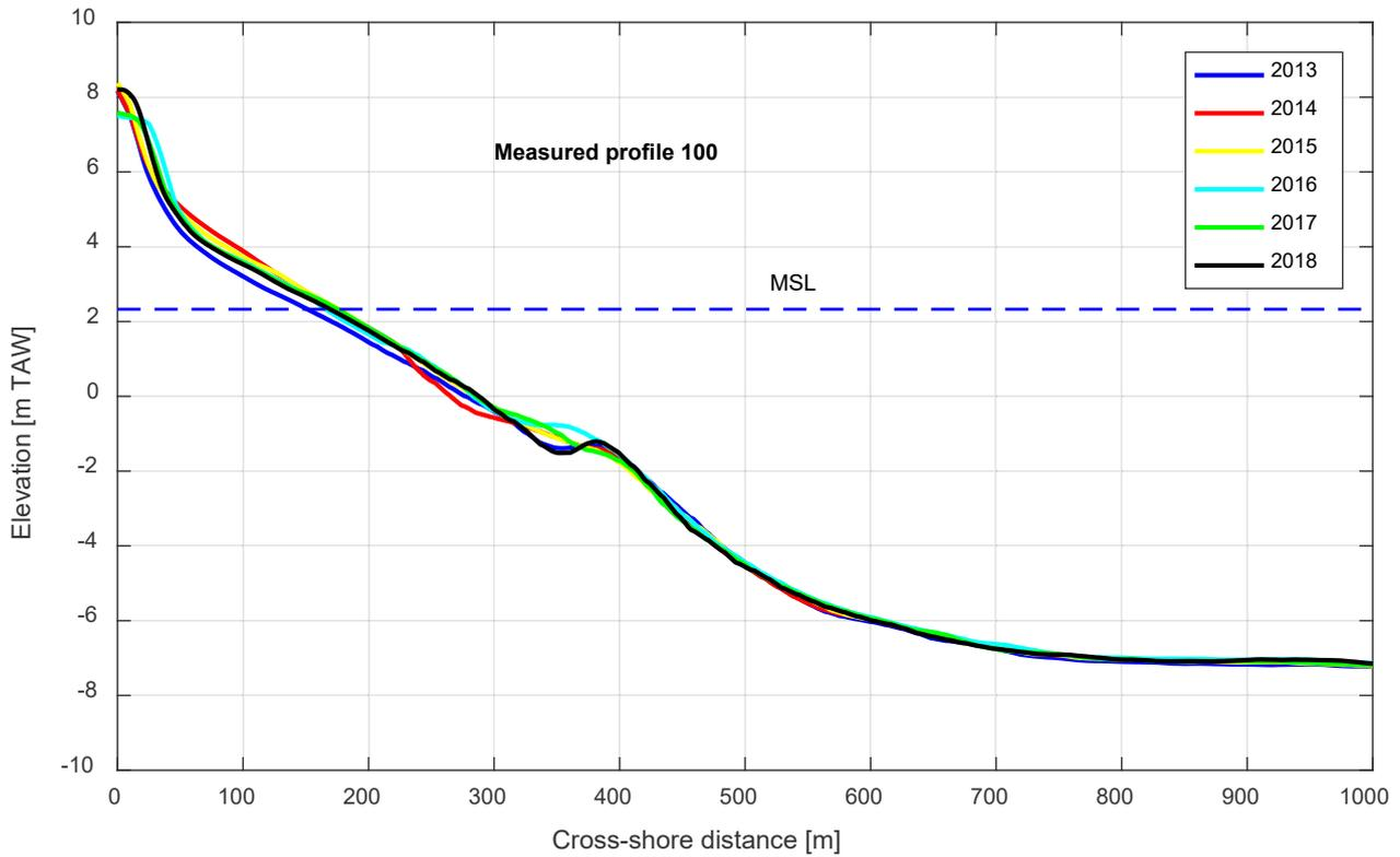
Figure 31 – Evolution of the cross-shore profile at Raversijde: profile 100.
