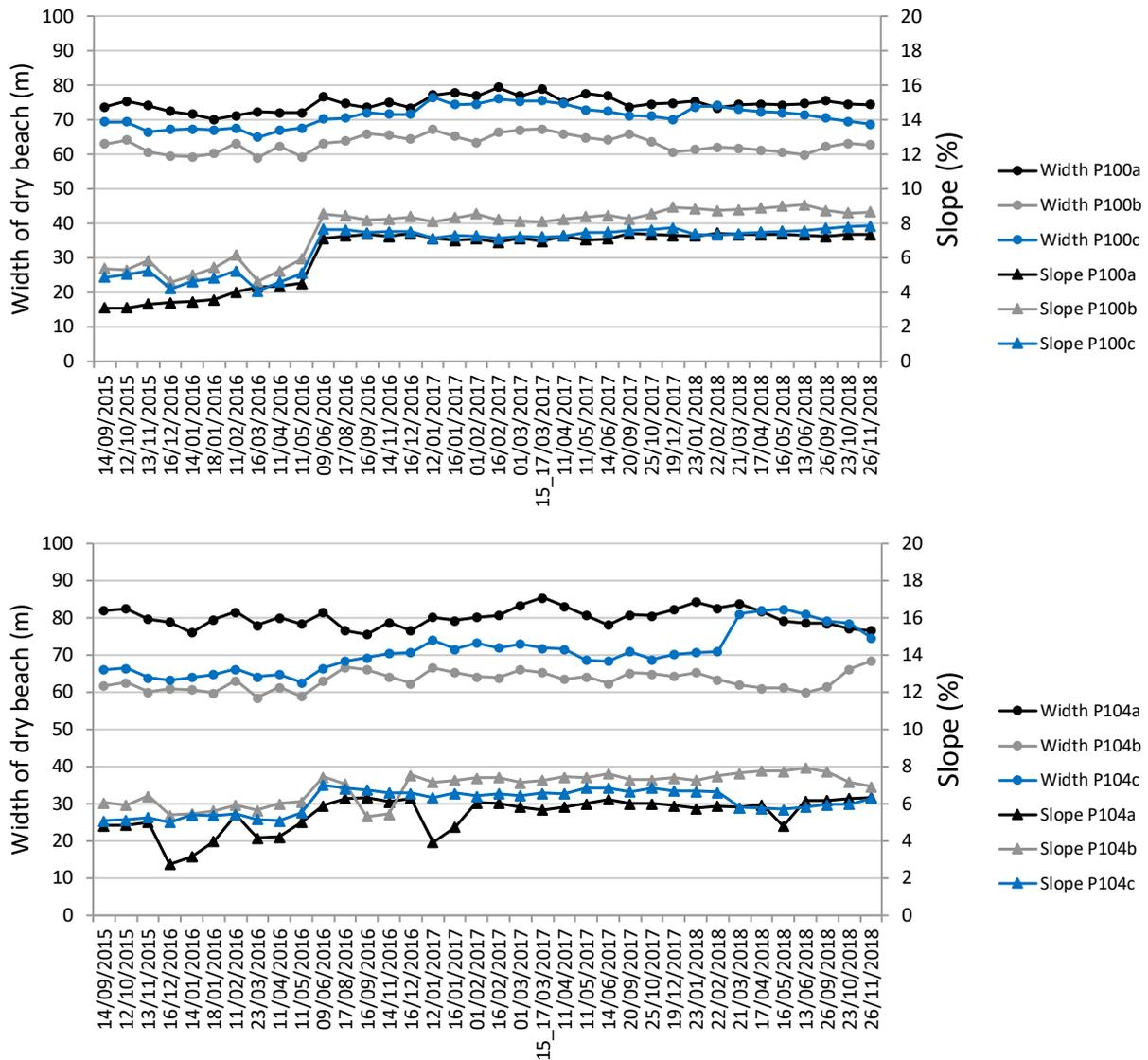
Figure 9 – Evolution of the dry beach width (slope) at Raversijde-East (section 100) and at Mariakerke (section 104).
