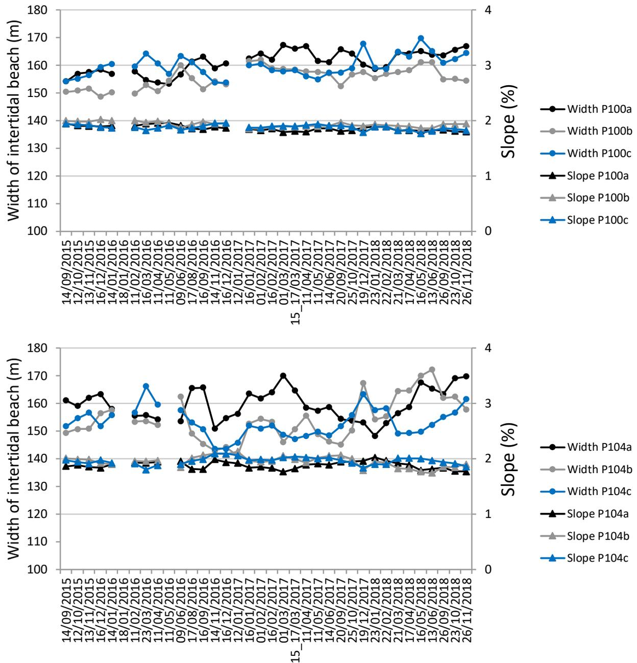
Figure 8 – Evolution of the intertidal beach width (slope) at Raversijde-East (section 100) and at Mariakerke (section 104).
