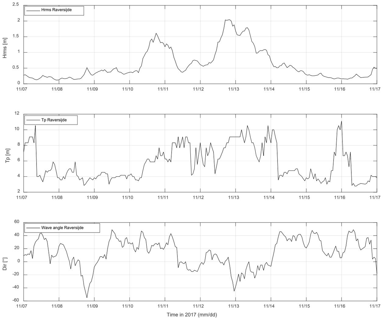
Figure 44 – Wave height, period, angle at Raversijde wave buoy used as boundary condition in UNIBEST-TC model.
