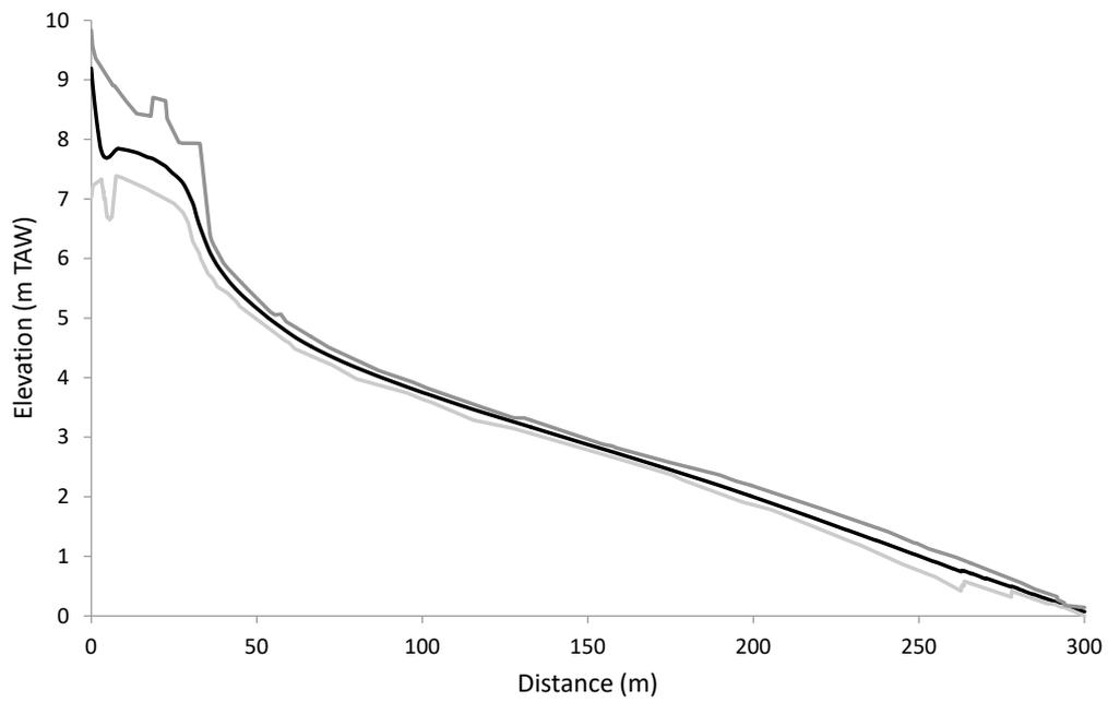
Figure 5 – Envelope of the cross-shore profiles for section P100 (a, b, c) at Raversijde-East from September 2015 to December 2017.
