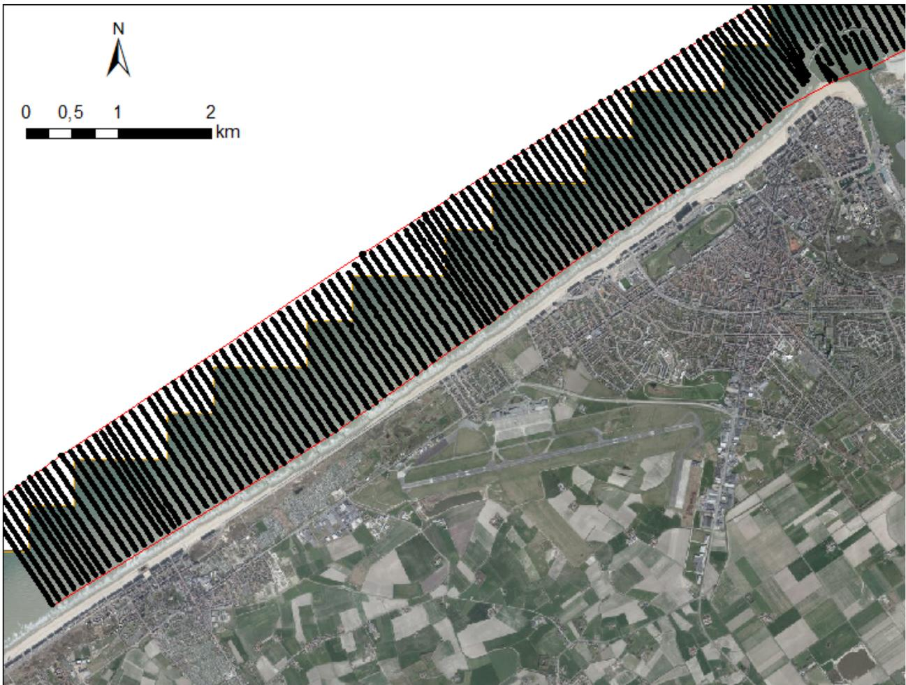
Figure 50 - Example of a single-beam dataset and the corresponding delineated polygon for the study area (survey conducted in 04/06//2015).
