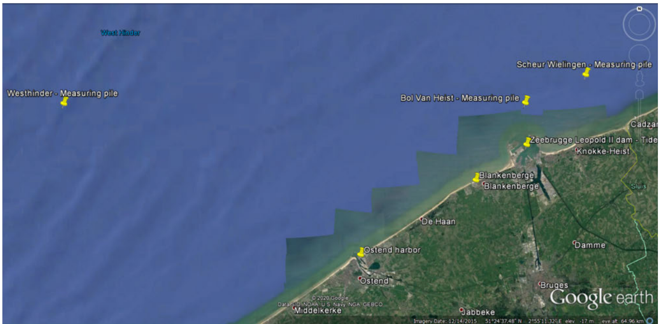
Figure 149 – Locations of the water level and current velocity measurement stations.
