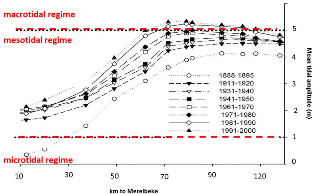
Figure 4-1: Evolution of the mean tidal amplitude (modified after Van Braeckel et al. 2006). Tidal range classifications based on Hayes (1979).
