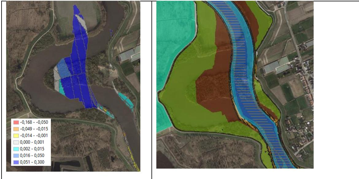
Figure 4-8: Example of extreme reduction in shear stress in VaG AplusCH as a consequence of a cut off bent: decrease of shear stress (TAU 50; blue coloured area in the left panel) in the high tidal mudflat (brown coloured area in the right panel).
