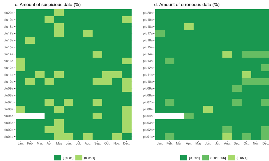
Figure 9: Illustration of the amount in % of suspicious and erroneous data per station and month. Erroneous values are those between 0mm and 50mm that had to be corrected.
