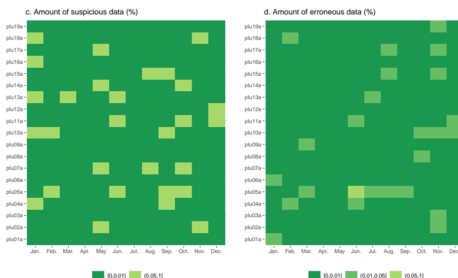
Figure 8: Illustration of the amount in % of suspicious and erroneous data per station and month. Erroneous values are those between 0mm and 50mm that had to be corrected.
