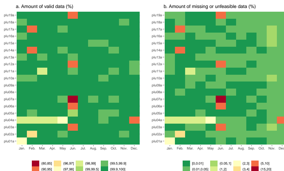
Figure 7: Illustration of the amount in % of valid and missing/unfeasible data per station and month. Unfeasible 5-min data are those with a negative value or a value larger than 50mm.
