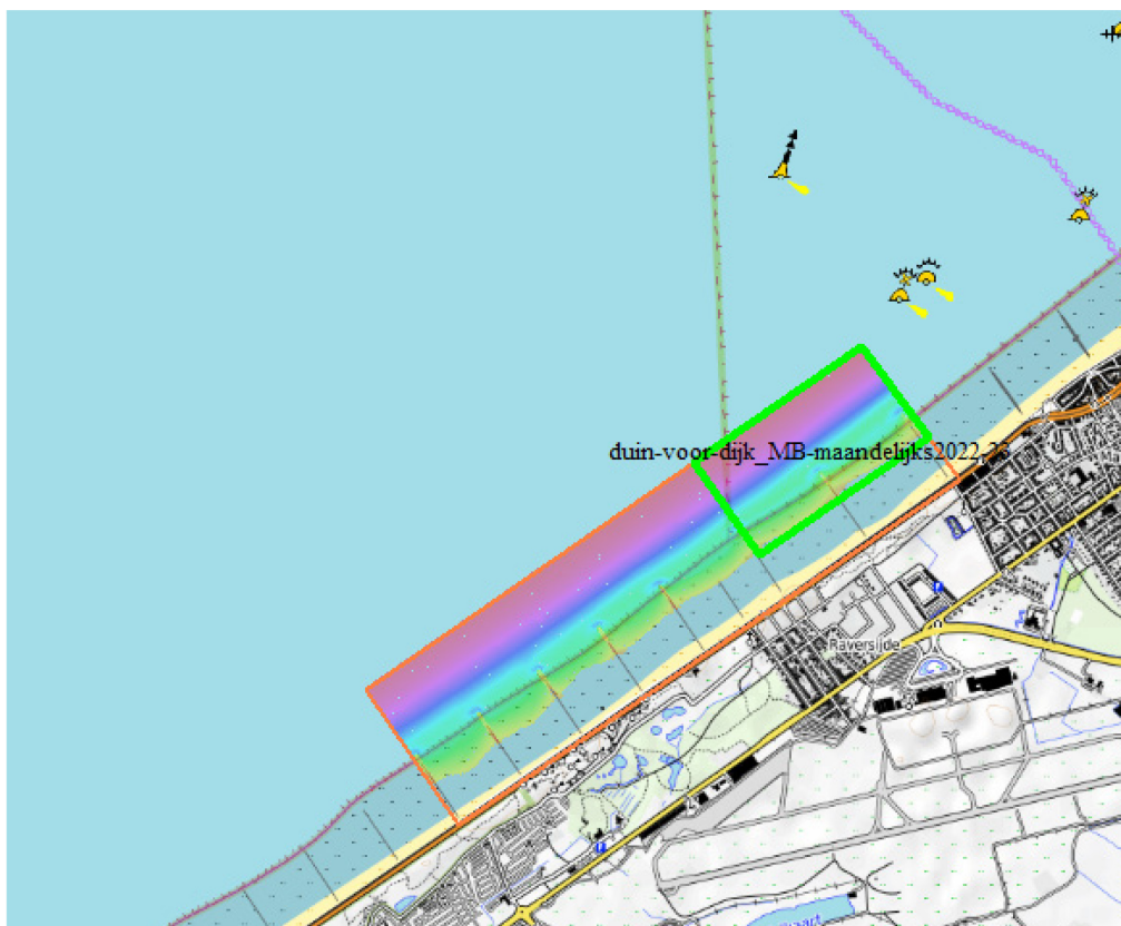
Figure 2 – Typical coverage of the large (red rectangle ) and reduced (green rectangle) multi-beam shoreface surveys
