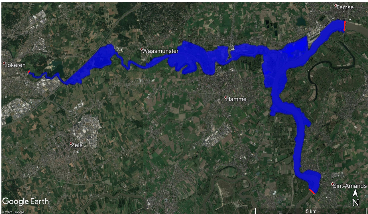
Figure 2 – The Durme model (blue) with three model boundaries (red) (Nguyen et al, 2024)
