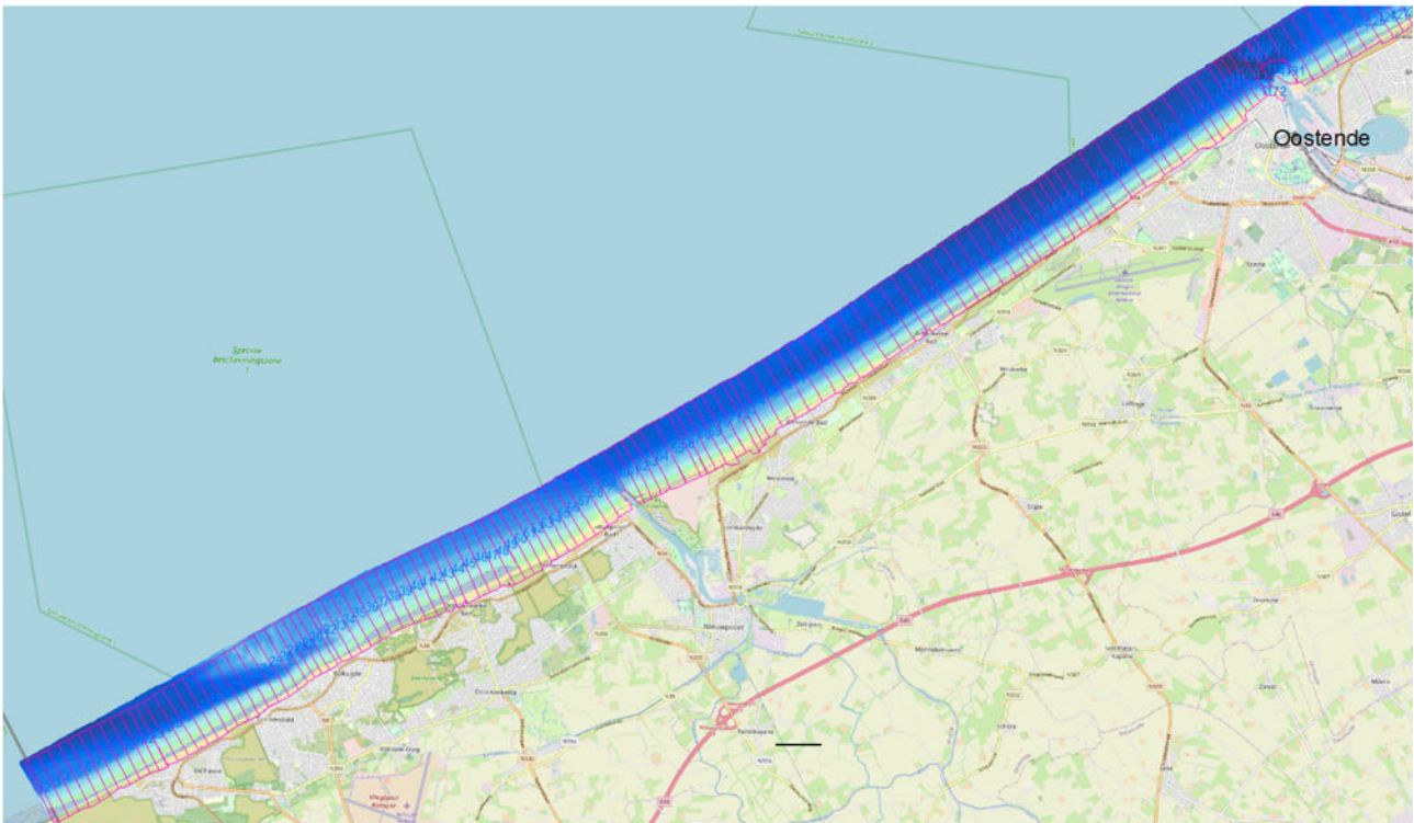
Figure 8 – 10 m-DEM of spring 1992 nearshore survey between French border and Oostende. Elevations range from about -8 to +1 m TAW.
