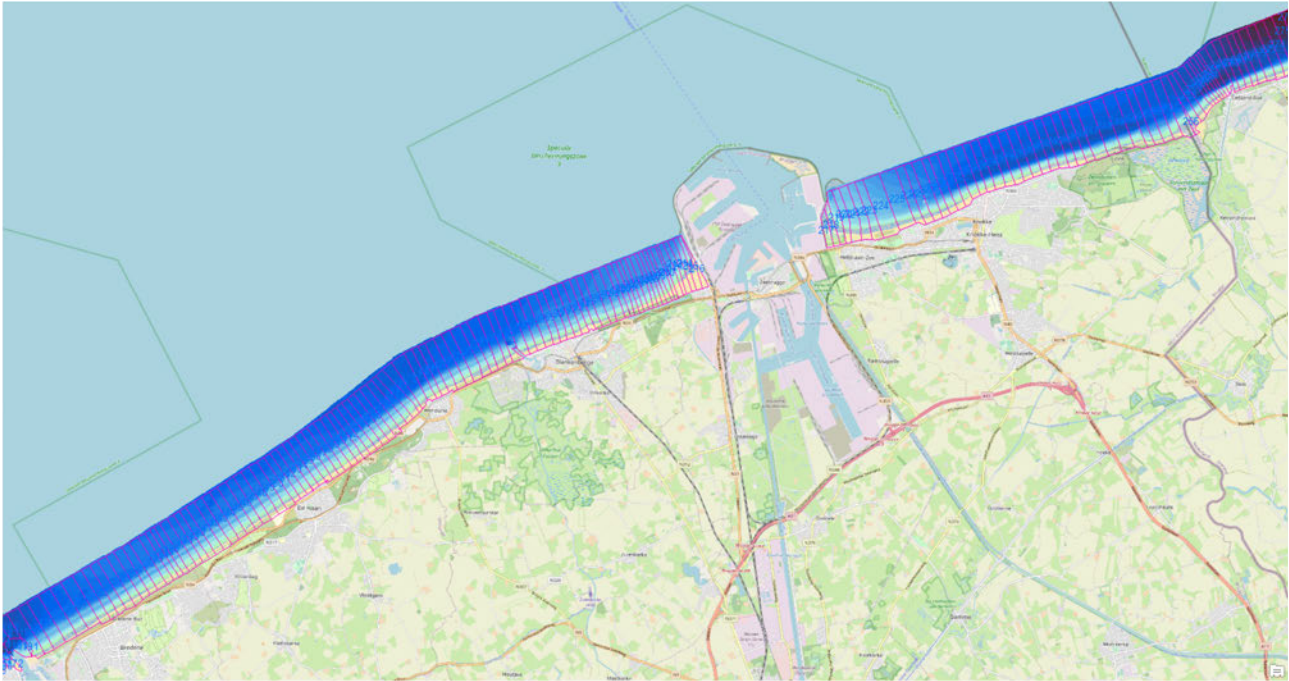
Figure 9 – 10 m-DEM of spring 1992 nearshore survey between Oostende and Cadzand. Elevations range from about -8 to +1 m TAW.
