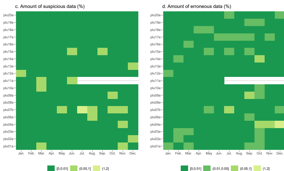
Figure 10: Illustration of the amount in % of suspicious and erroneous data per station and month. Erroneous values are those between 0mm and 50mm that had to be corrected.
