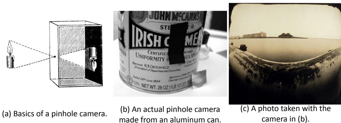
Figure 4 – pinhole camera and source of distortions (source: google.com).
