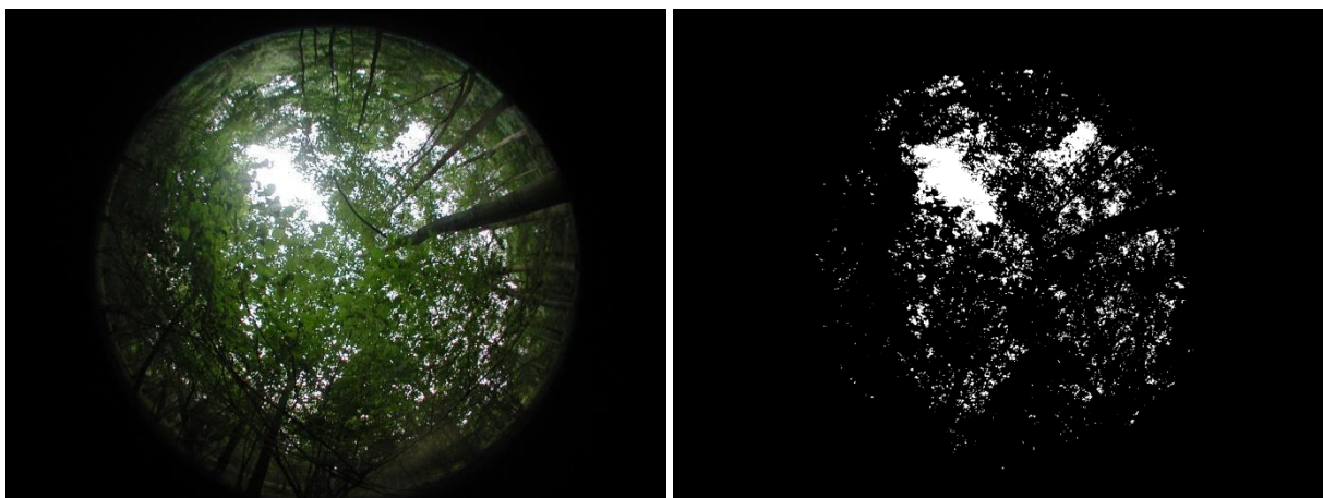
Fig. 11. Result of fisheye photography: left = original image; right = binary image for visual sky to derive gap share and LAI
