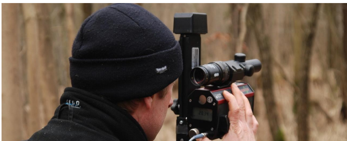
Fig. 7. FieldMap measurement configuration showing telescopic sight, Laser Forest Pro (below) and Mapstar digital compass (vertical box-shaped device on the left).
