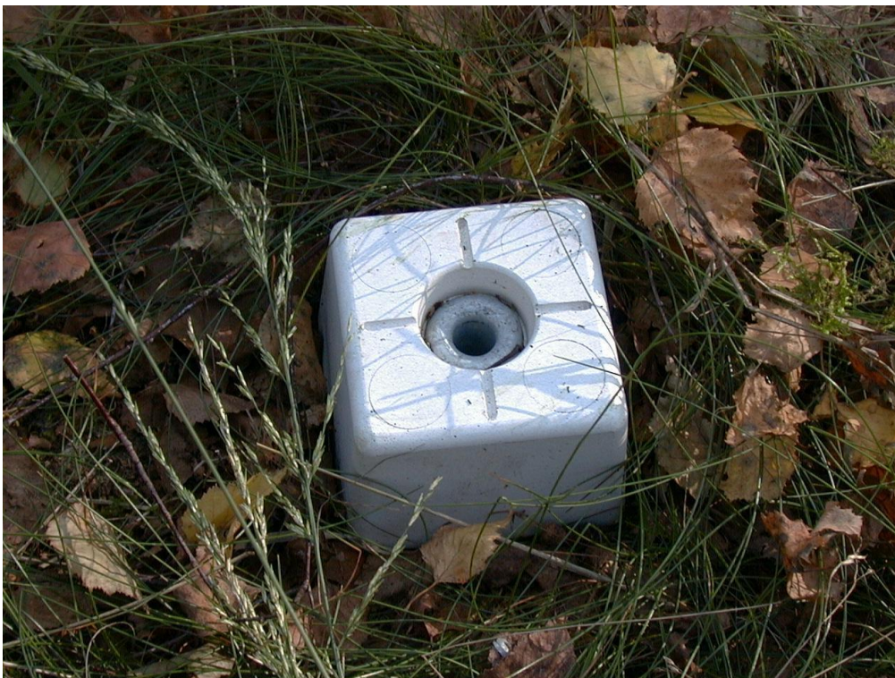
Fig. 5. A Feno marker is used to indicate the plot centre (photograph by Bruno De Vos)
