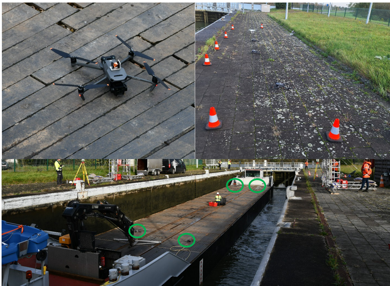
Upper left: 360° mini prims mounted on drone / upper right: landing area drones lower: positioning drones on the ship deck indicated by green circles
