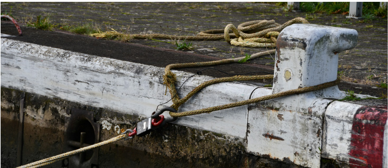
Figure 12 - Load cell mounted in between mooring line and lock platform bollard
