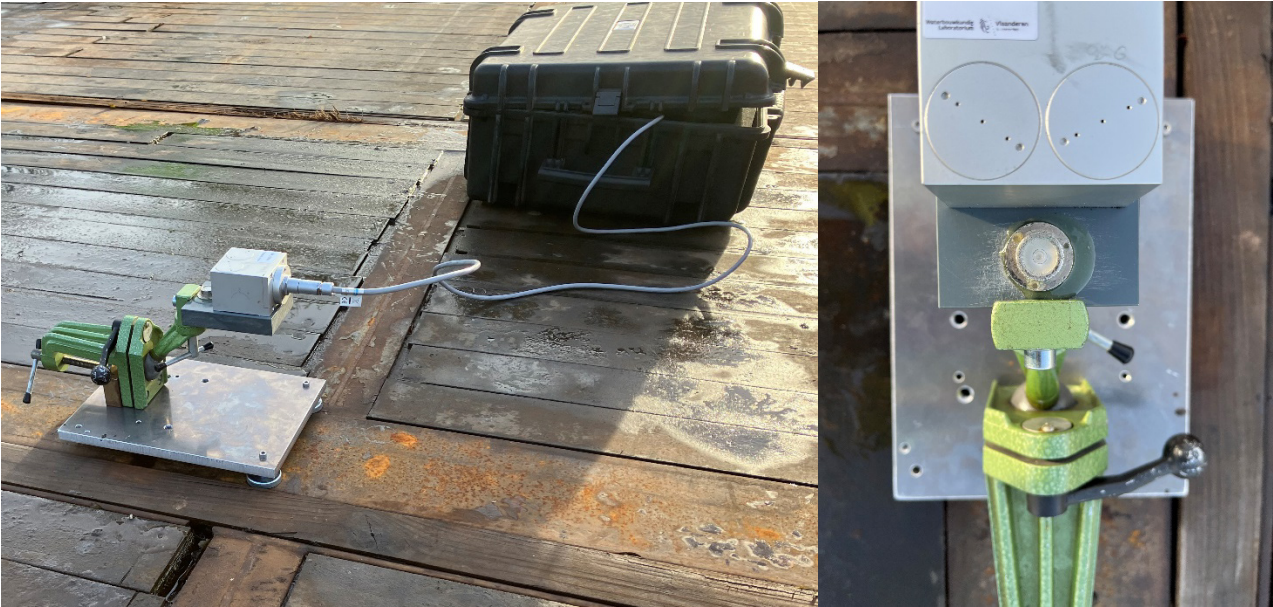
Figure 9 - Inclinometer mounted on deck Zulu I during PoC Iv-Infra
