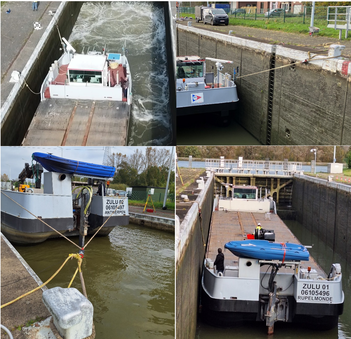
Upper left: PoC Apixa / Upper right : PoC Iv-Infra positioned upstream Lower left: PoC Apixa mooring line controlled by winch / Lower right : PoC Iv-Infra mooring manually controlled
