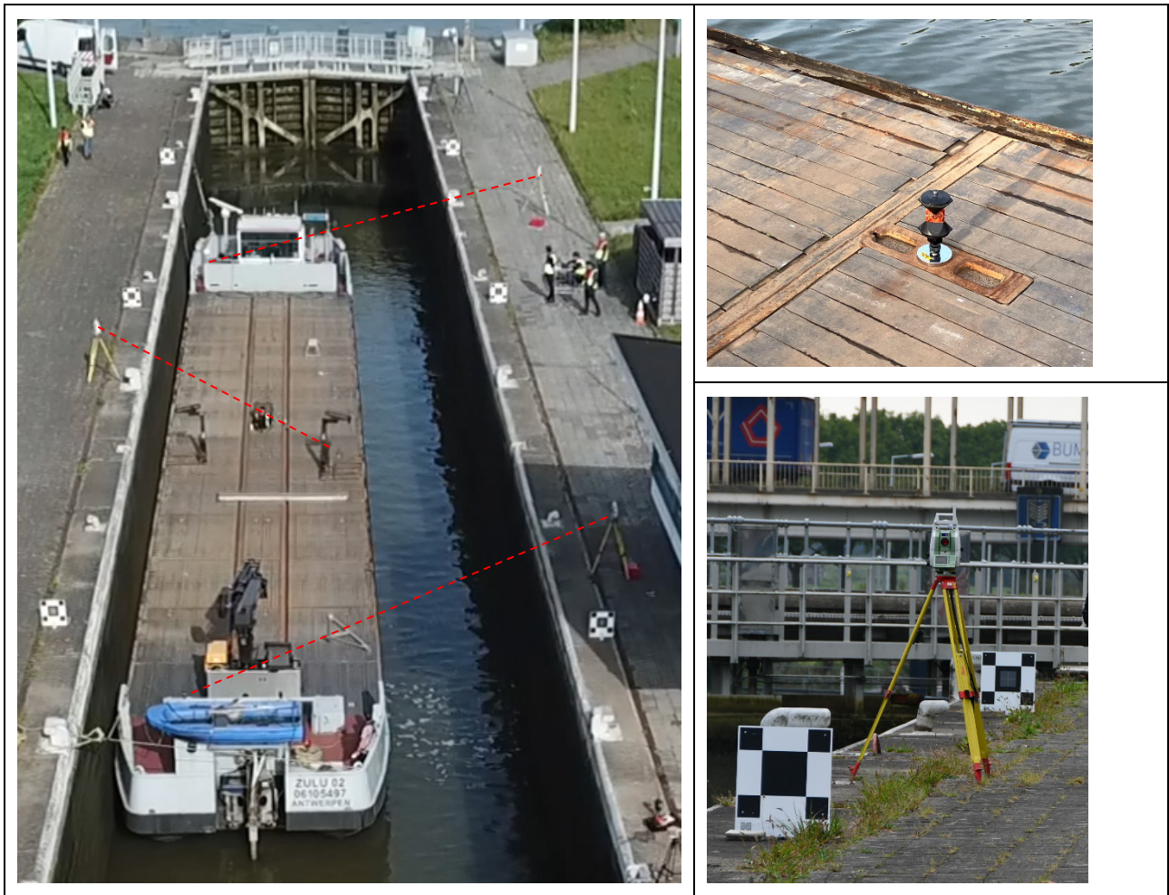
Left : Set-up tachymeters tracking each a prism Upper right: prism / lower right: tachymeter
