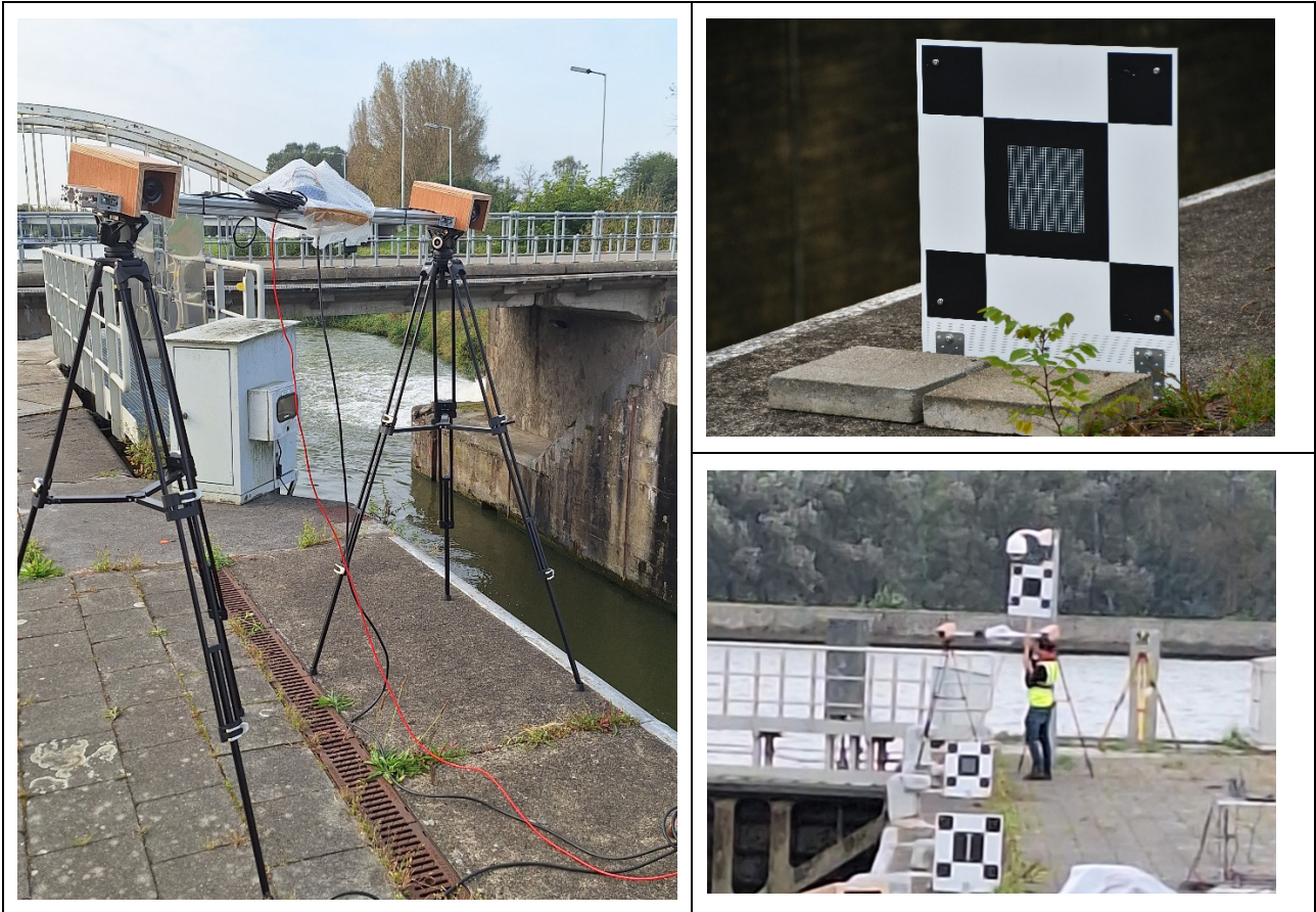
Left: stereo pair; upper right: fixed marker; lower right: free moving-marker
