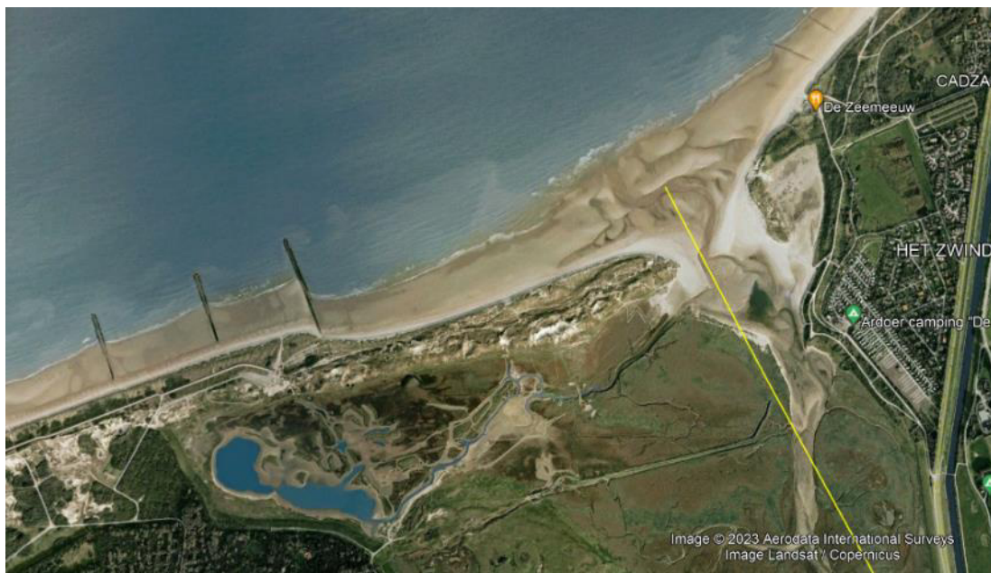
Figure 46. Google Earth image of the effect of the most eastward groyne.
