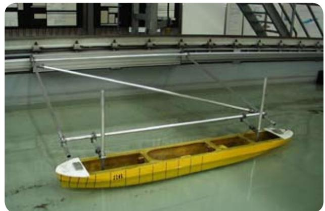
Auxiliary carriage for ship interaction tests
