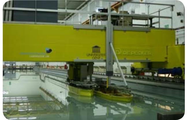
Ship-ship interaction tests: Aframax and VLCC
