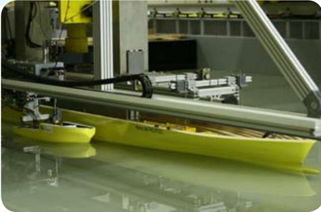
Ship interaction tests: tugboat and Container ship.
