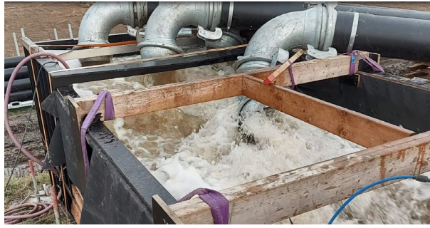
Figure 8 – Emitting of water from the supply tubes to the water surface during the third test period
