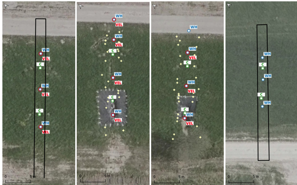
Figure 24 - Position of sensors and portals during B-OF08 (left), B-OF10, B-OF11 and N-OF03 (right) - WH=water height sensor, VEL=point velocity meter, C= control point
