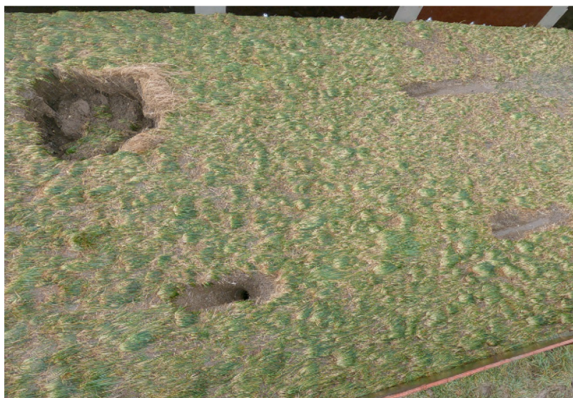
Figure 49 – Erosion pit around pipe inlet in box 7-8CD during the N-OT04 test (15' after start of wave set III)
