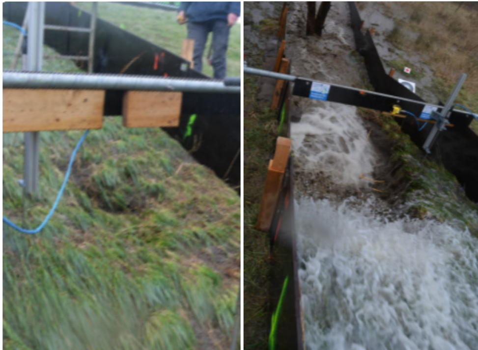
Figure 34 - Depression of the cover layer before the last run (left) and the collapse and erosion afterwards (right) during test B-OF11 (Photos: A. Koelewijn).
