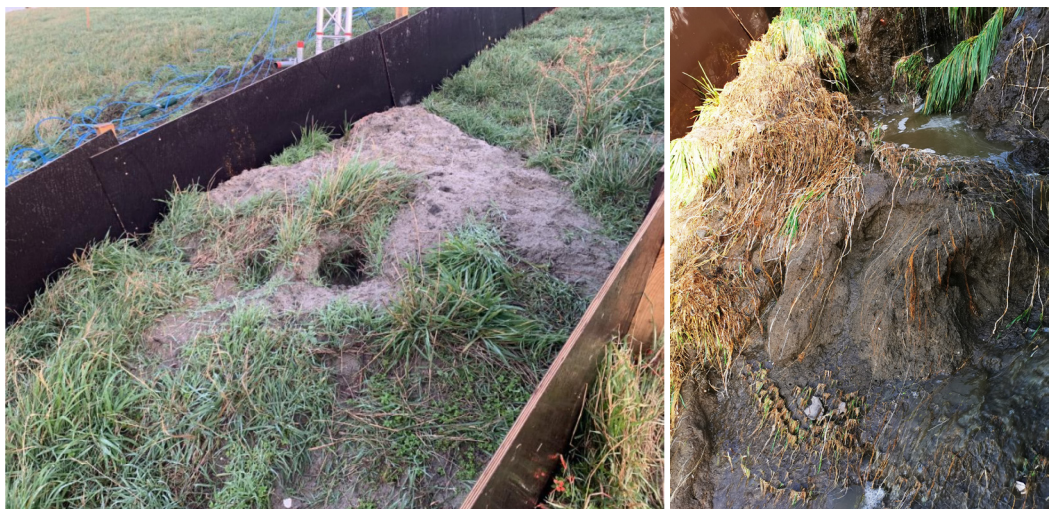
Figure 27 – N-OF05: (left) initial burrow state and (right) exposure of wire fence (lower part of the image) and erosion depression (upper part of the image) during the experiment.
