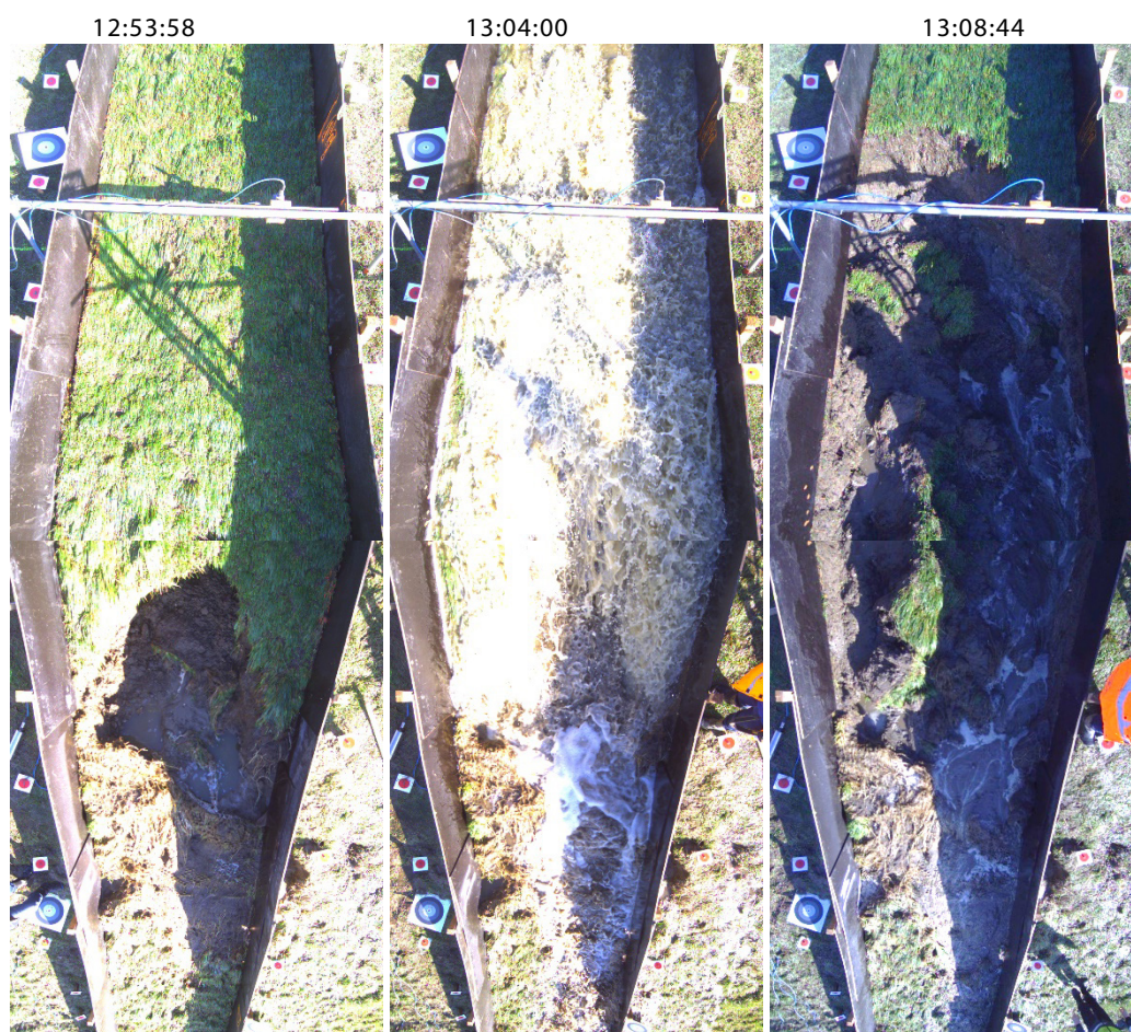
Figure 28 - N-OF05: Evolution of the damage during the last 15 minutes of the test; upper camera portal (= upper slope view).
