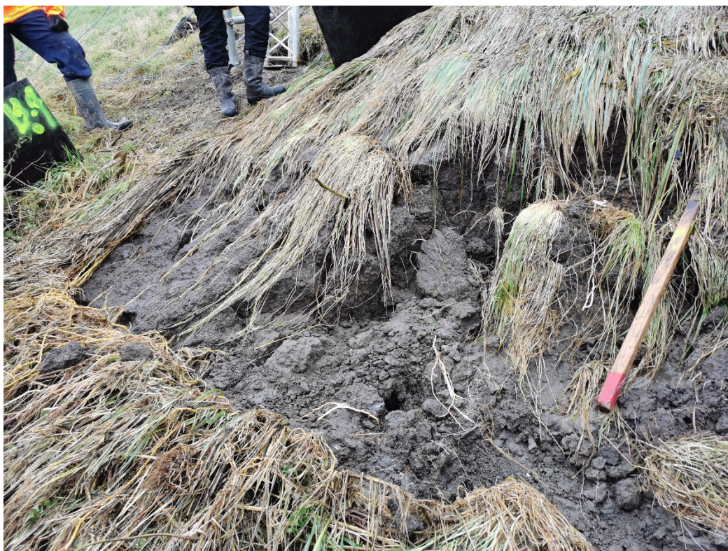
Figure 40 - Detail of the damage on the upper side of the reed field after 30 minutes of overflow.
