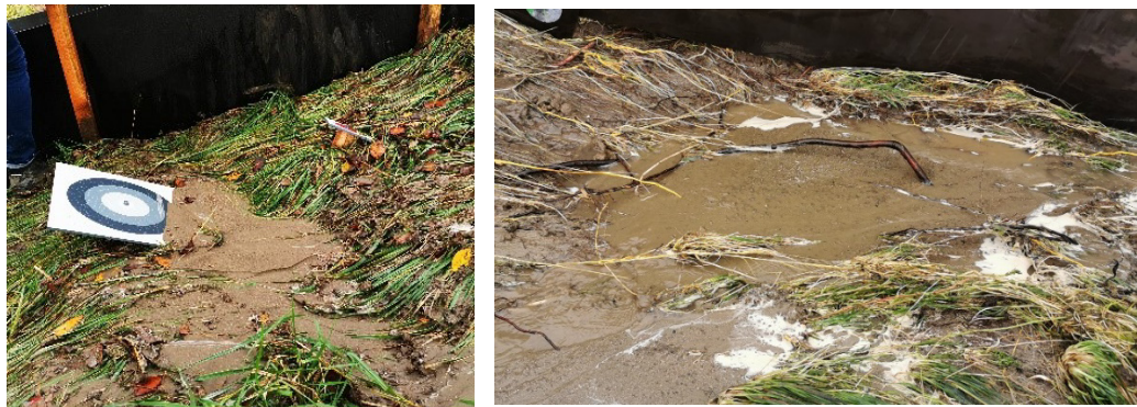
Figure 29 - Sand outflow and boils outside the test section (left: B-OF04 outside the section; right: B-OF11 inside the section).
