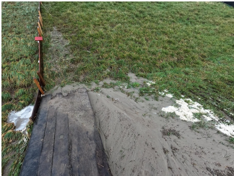
Figure 43 - Sand released through a mole hole outside the test section after 4 sets of waves.
