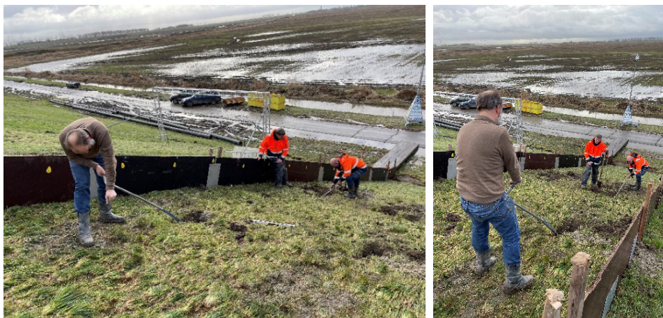
Figure 48 – Drilling of 2 adjacent burrows during test N-OT04 with inlet in box 7-8AB/CD and outlet in box 13-14AB/CD
