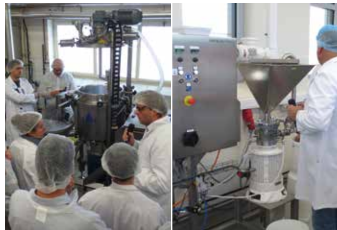
Preparation of mayonnaise with the high shear mixer in the Food Pilot
