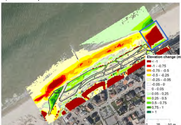
Figure 23 – Global evolution based on DoDs of the UAV and LiDAR surveys at Westende. The changes of the building (landward of the seawall) are artefacts.
