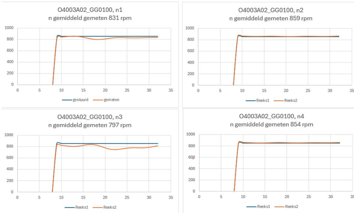
Figure 5-1 : Analysis of DPT output (RES->DPT) of test O4003A02\_GG0100 for the four propellers.
