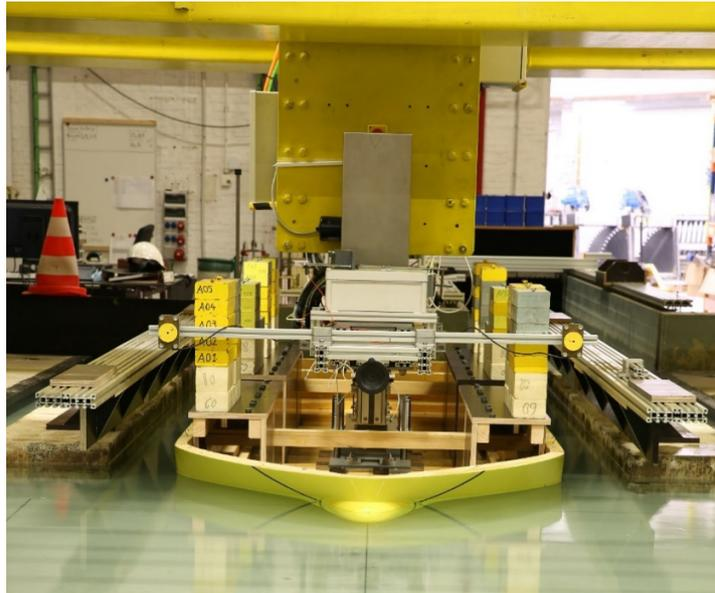
Figure 4-1 : Photo temporary harbour set-up for test campaign O40.
