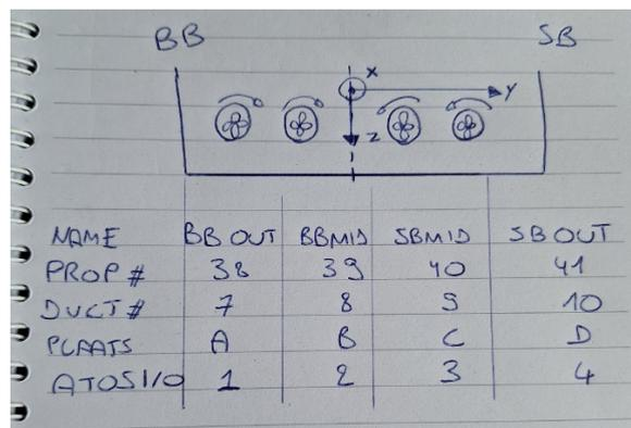
Figure 4-3 : Definitions appendages as used in the Towing tank Tests for ship O40
