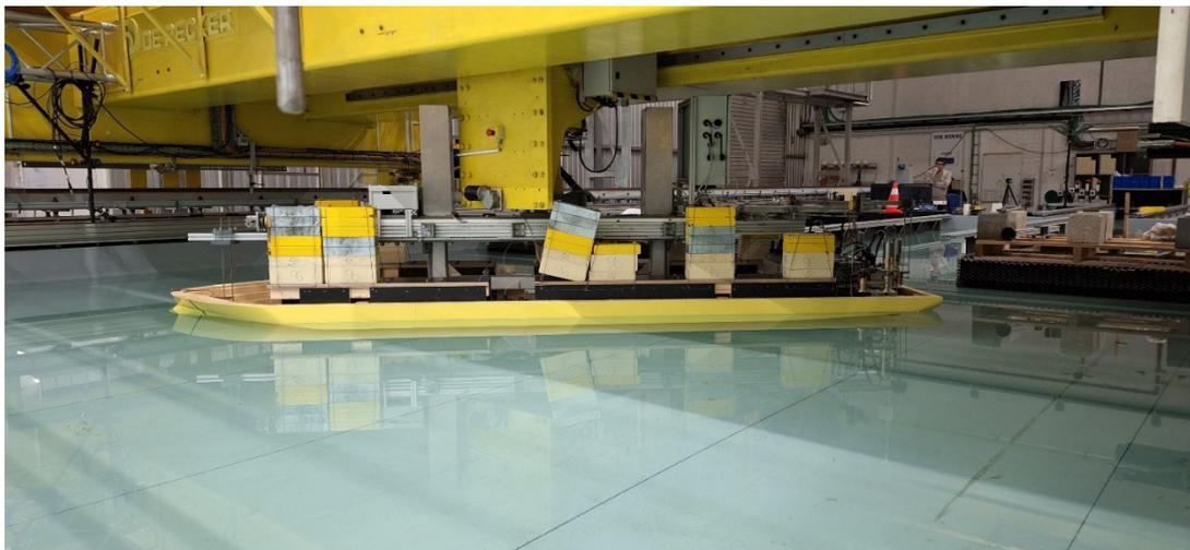
Figure 12-1 : Interference between the weights distribution and the carriage structure.
