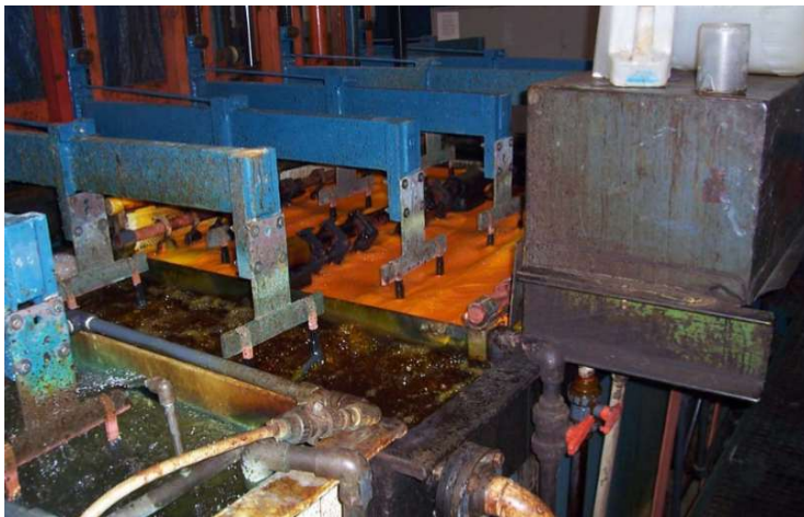
Figure 12 : Chroming-plating bath (with orange foam) with rinse baths (EPA, 2009)
