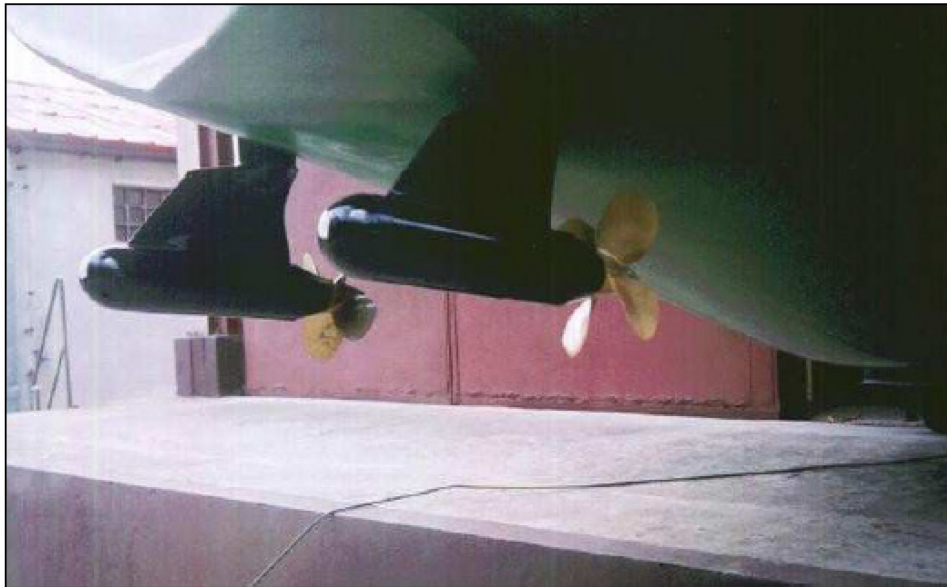
Figure 3 – Ilawa training model of a large LNG carrier equipped with two azipods
