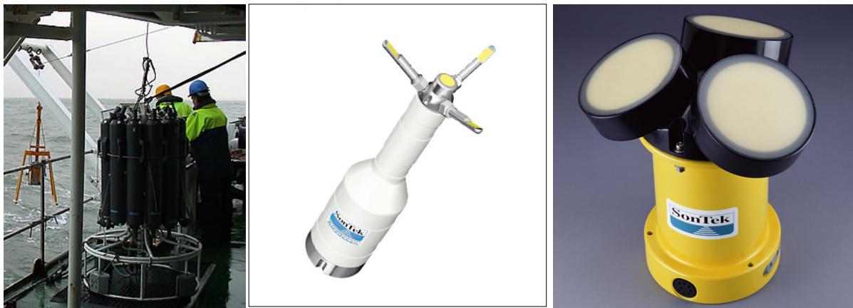
Figure 2 - Niskin Carrousel (left), SonTek ADVOcean sensor (middle) and SonTek ADP (right)
