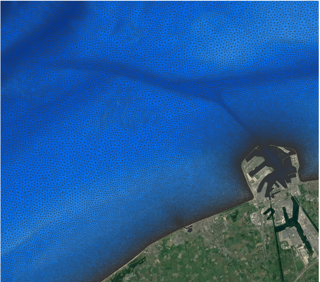
Figure 4 – Detail of the ScaldisCoast grid in the surrounding of Zeebrugge
