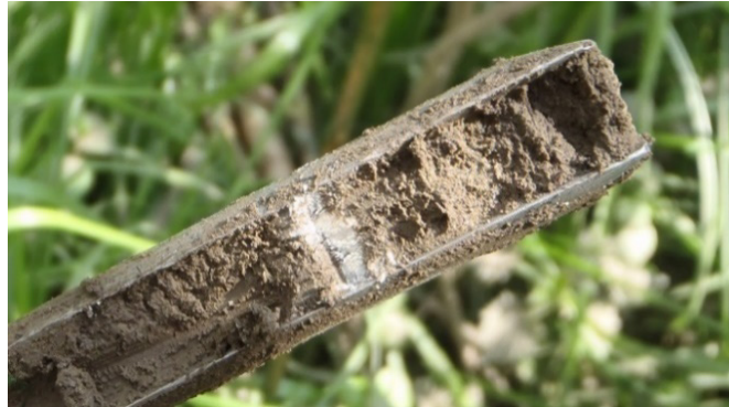
Figure 48 - Marker Horizon using a white kaolin clay layer (Maris et al, 2023)
