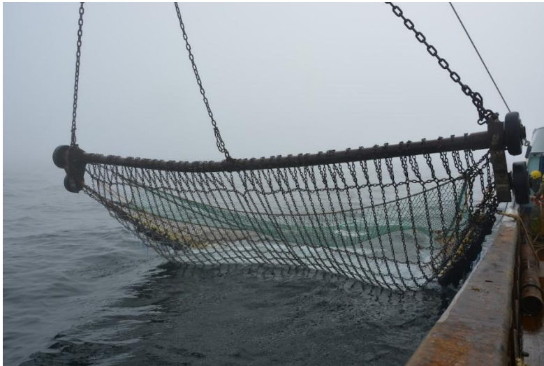
Figure 4-4 Beam and chain mat used during the PreciVis survey. Picture taken during the survey (16/04/2025).
