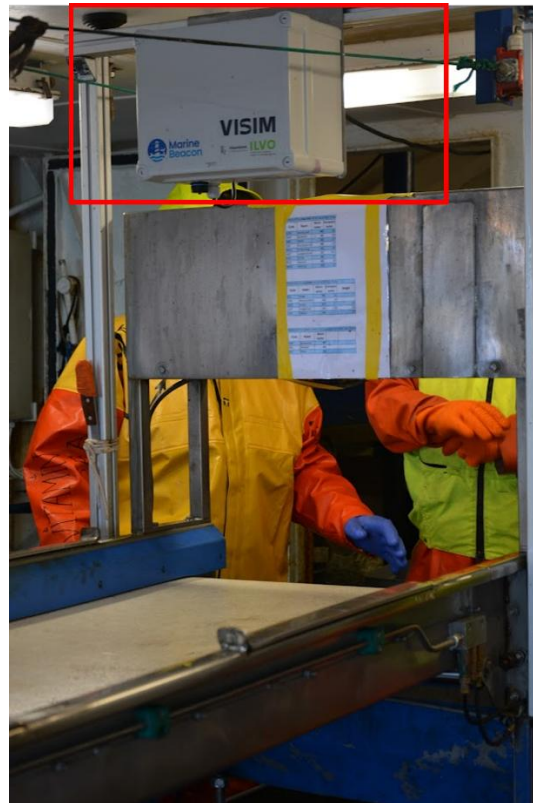
Figure 5-3 VISIM camera installed on the survey vessel (Z.510-Dennis) during the PreciVis survey (red).
