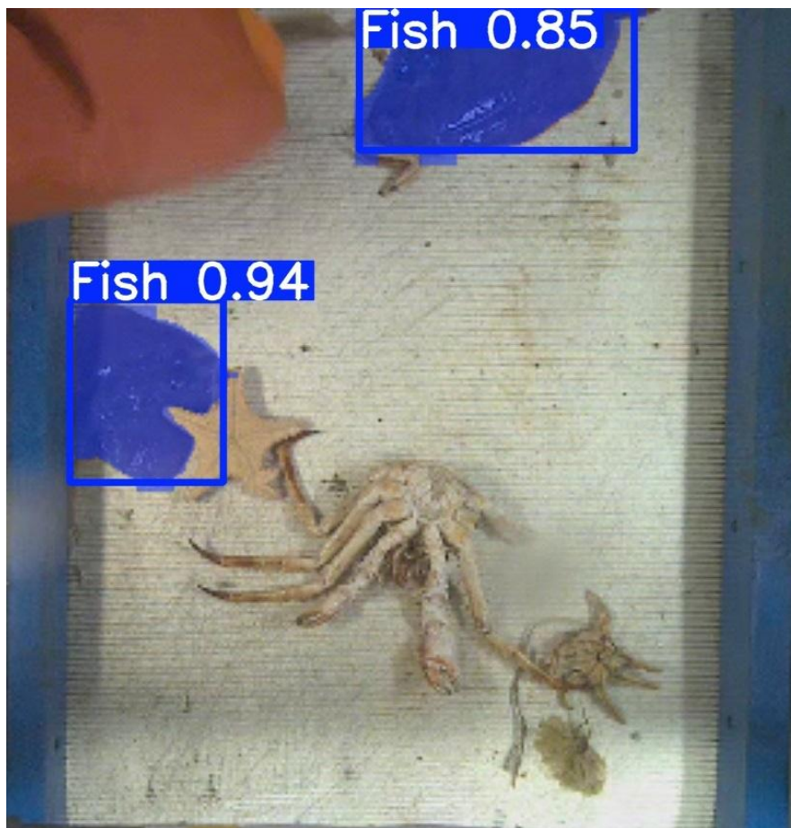
Figure 13-2 Processed image of Figure 13-1 . The search area is minimized, and fish species are detected. The number next to "Fish" represents the confidence of the prediction (maximum of 1).
