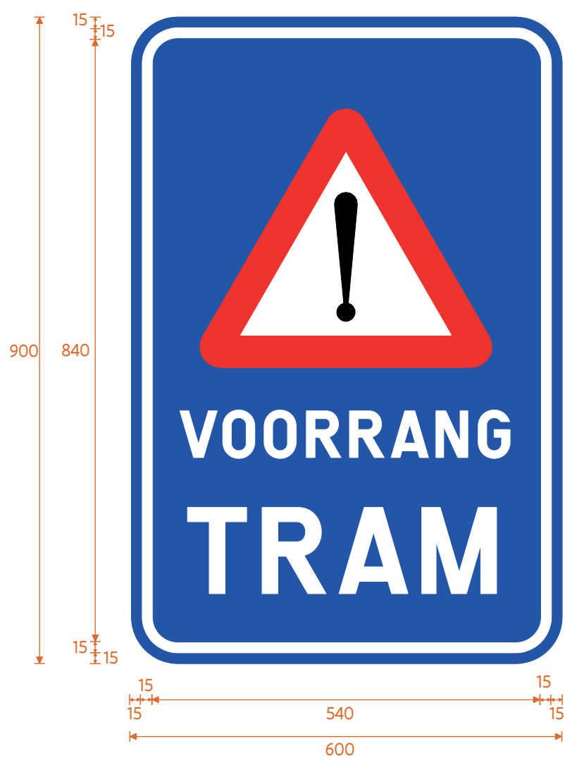
Details bord “voorrang tram” (in mm)
