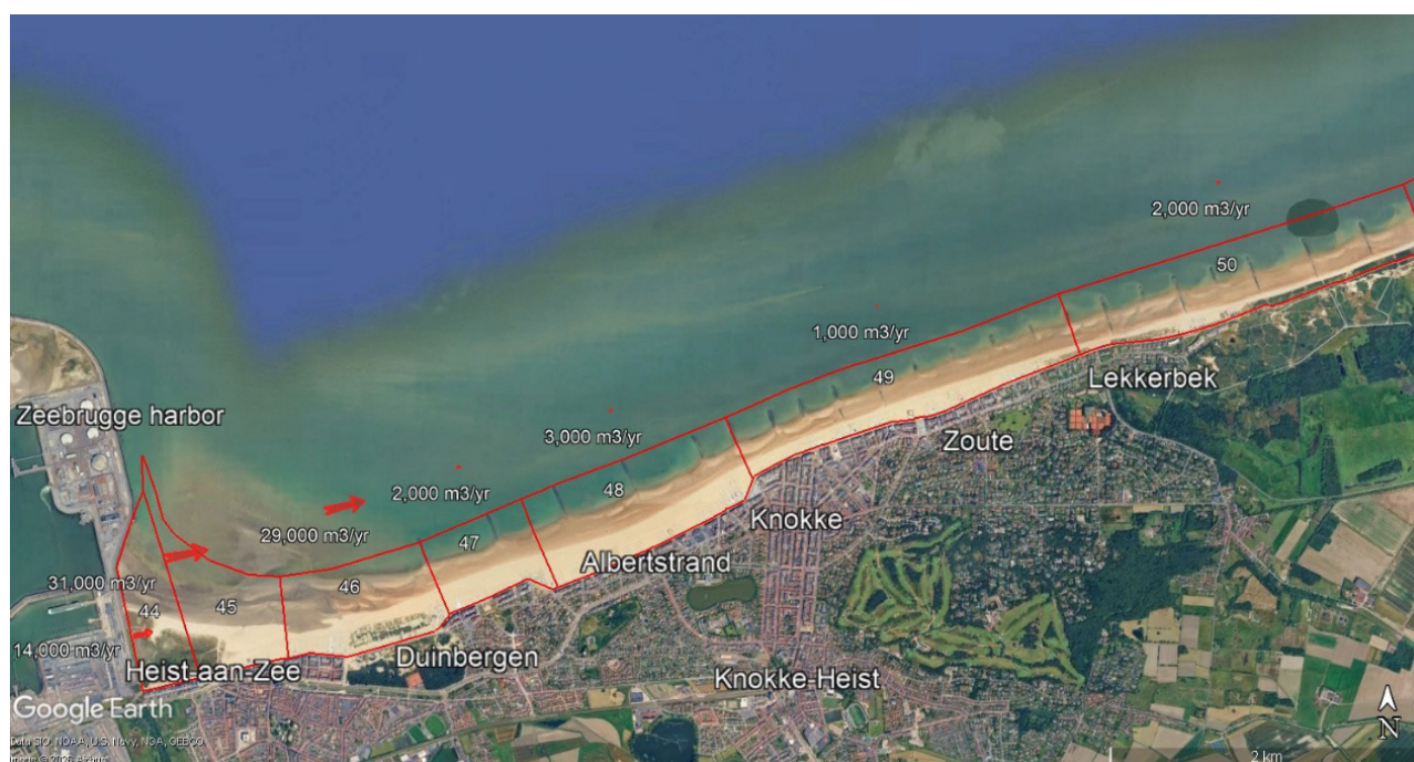
Figure 3-86: Longshore sediment transport magnitude and dominant direction per Strook over the calibration period 1983-1999, for simulation #6 with emerged groynes.
