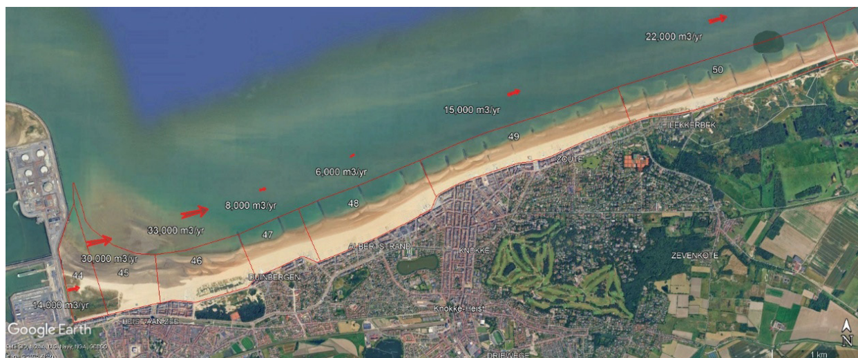
Figure 3-83: Longshore sediment transport magnitude and dominant direction per Strook over the calibration period 1983-1999, for the calibrated model, simulation #3 (with wave calibration of the eastern two locations).
