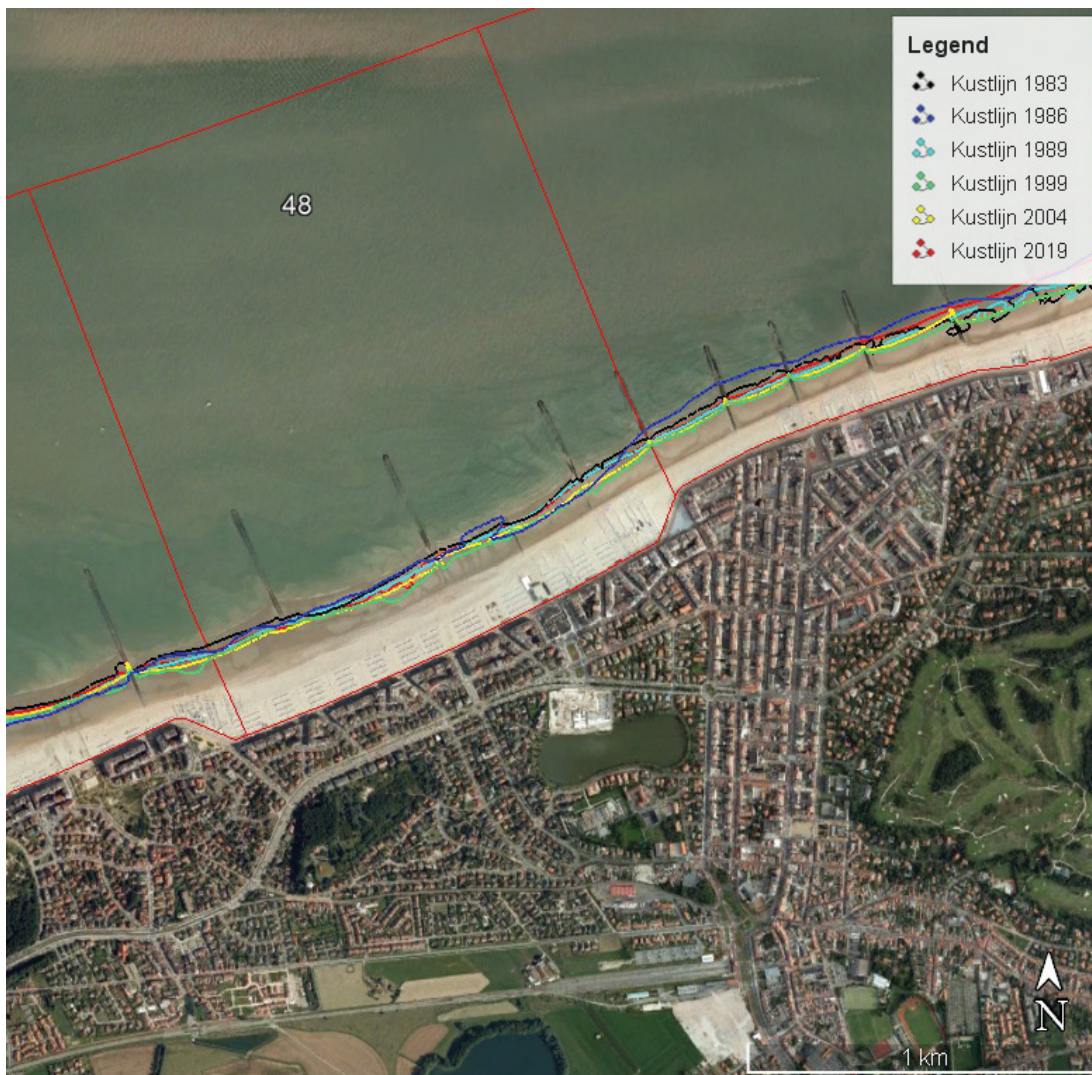
Figure 3-90: Coastline position for Albertstrand, Stroom 48, over time of the 2.33 TAW depth contour corresponding to mean sea level.
