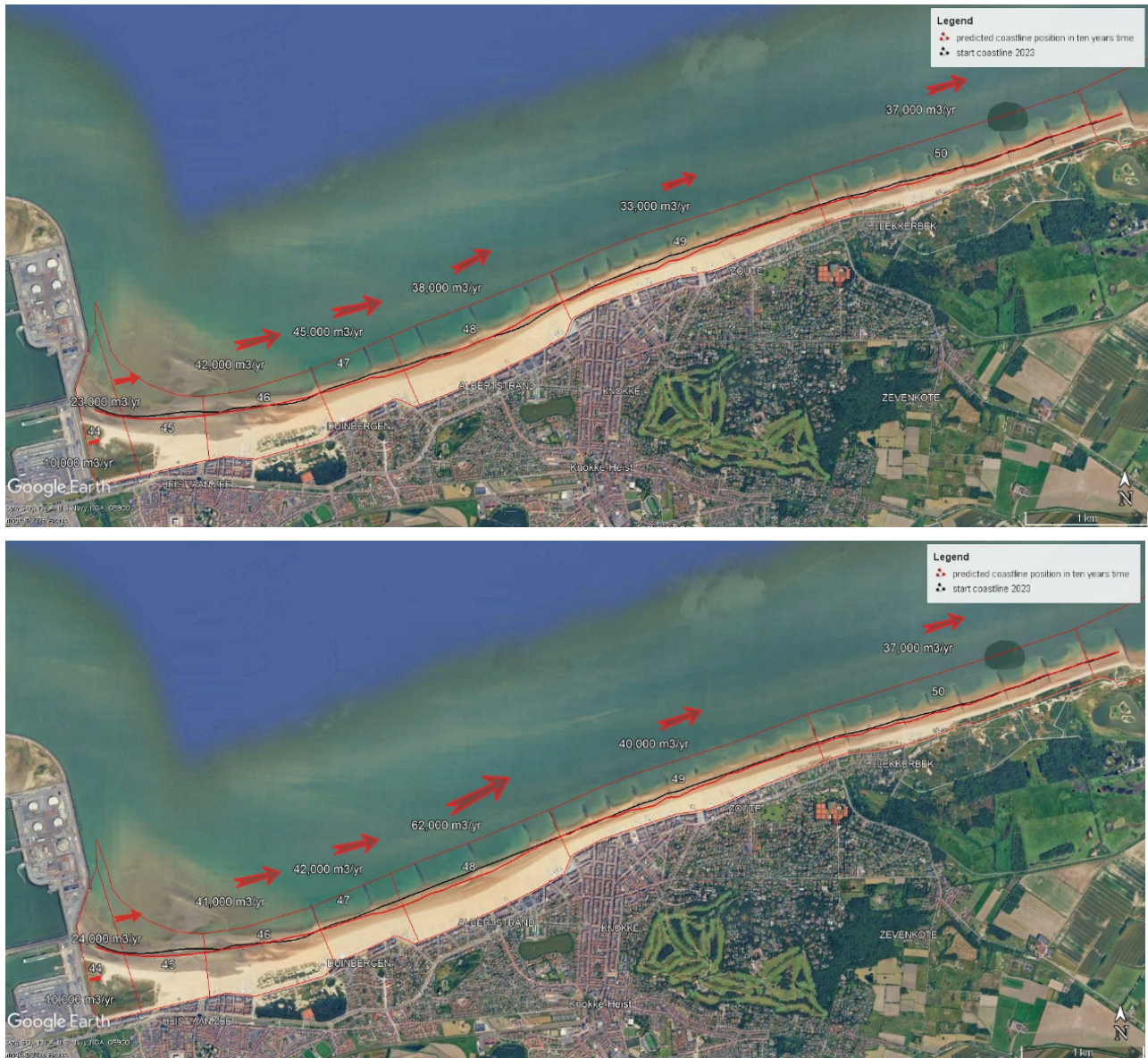
Figure 3-92: Longshore sediment transport magnitude and dominant direction per Strook for the calibrated model settings, for (top) simulation #13, reference coastline in 2023, (bottom) simulation #14, coastline in 2023 including Albertstrand nourishment scenario with straightening of the coastline.
