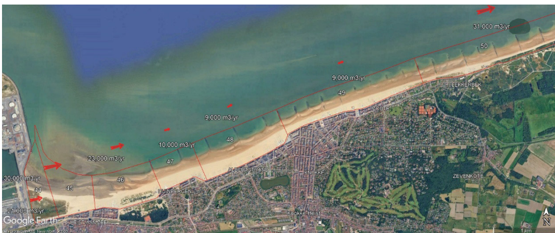
Figure 0-4: Longshore sediment transport magnitude and dominant direction per Strook over the calibration period 1983-1999, for simulation #5 with wave climate of Trouw et al. (2024).
