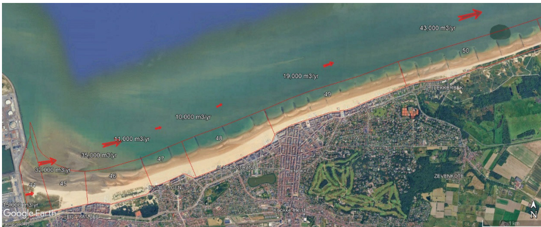
Figure 0-3: Longshore sediment transport magnitude and dominant direction per Strook over the calibration period 1983-1999, for simulation #1.
