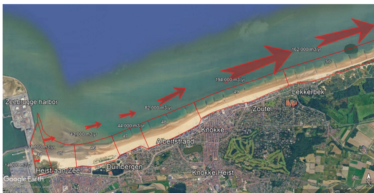
Figure 3-87: Longshore sediment transport magnitude and dominant direction per Strook over the calibration period 1983-1999, for simulation #8 without groynes.
