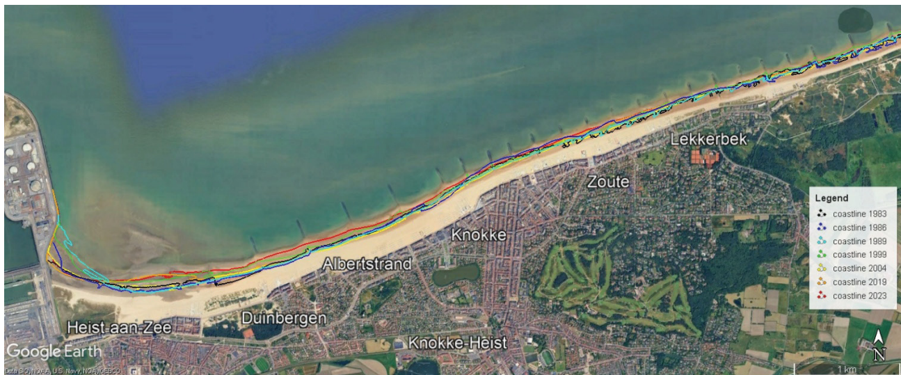
Figure 3-72: Coastline position over time of the 2.33 TAW depth contour corresponding to mean sea level.
